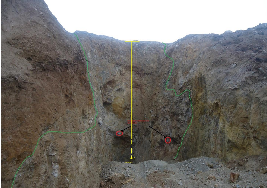
Cross-cutting exploration excavation: the altered zone (green border) coming up through the limestone with in-situ Pb (red circles)
