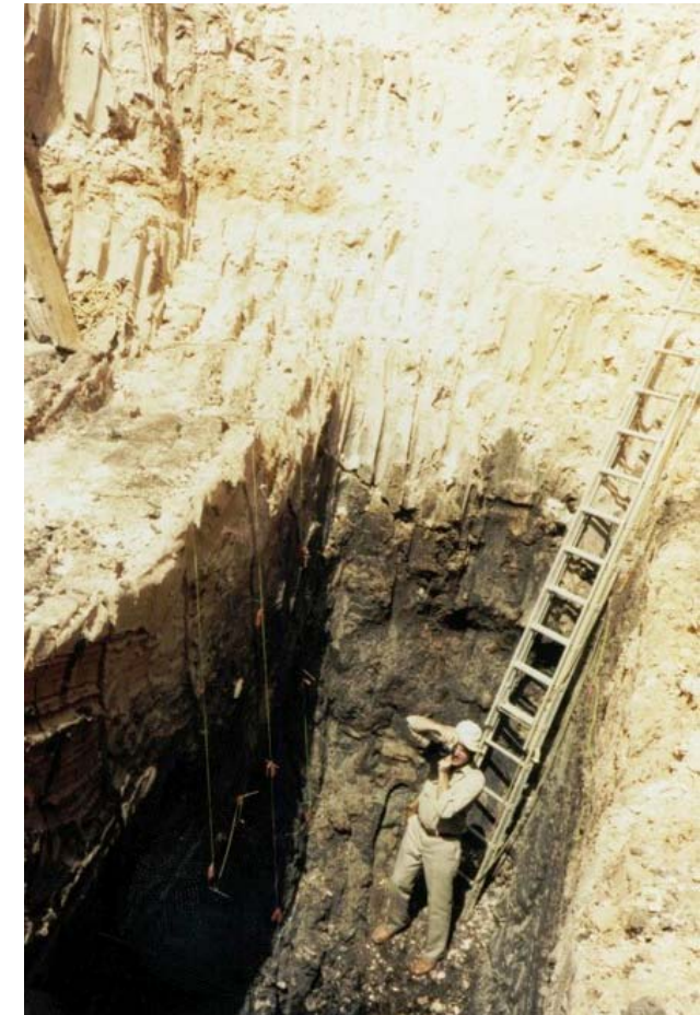
Close-up in test pit showing lignite ore and free dig nature of material
