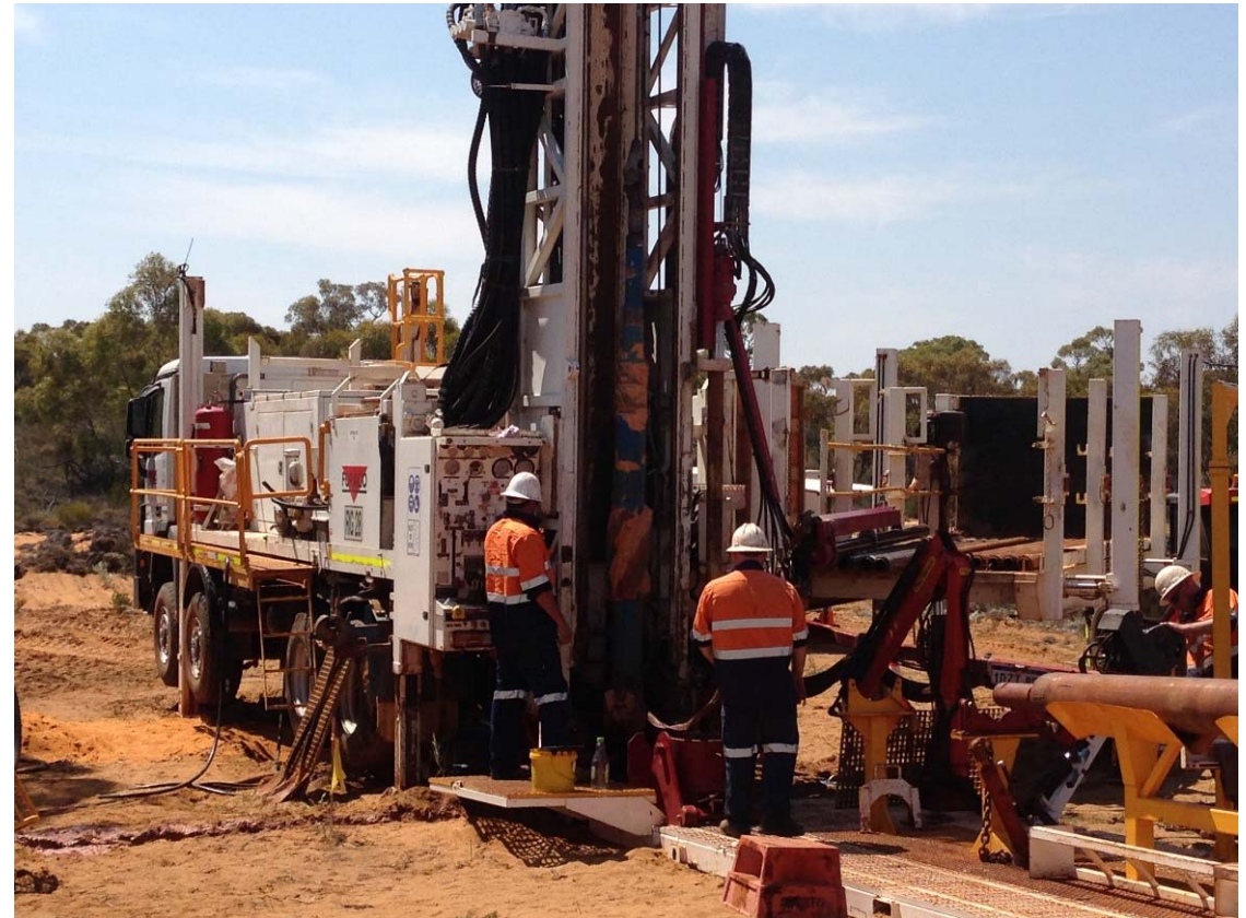
Metallurgical bulk sample drilling using 8" diamond core
