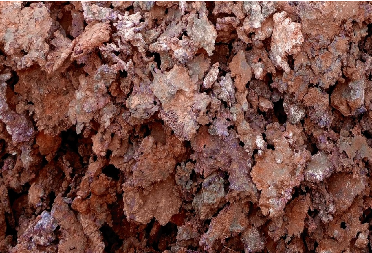
Figure 1: High-grade DSO (+40mm) visually estimated at 80-90% Cu, scalped off the crusher screens and loaded into containers ready for shipment.
