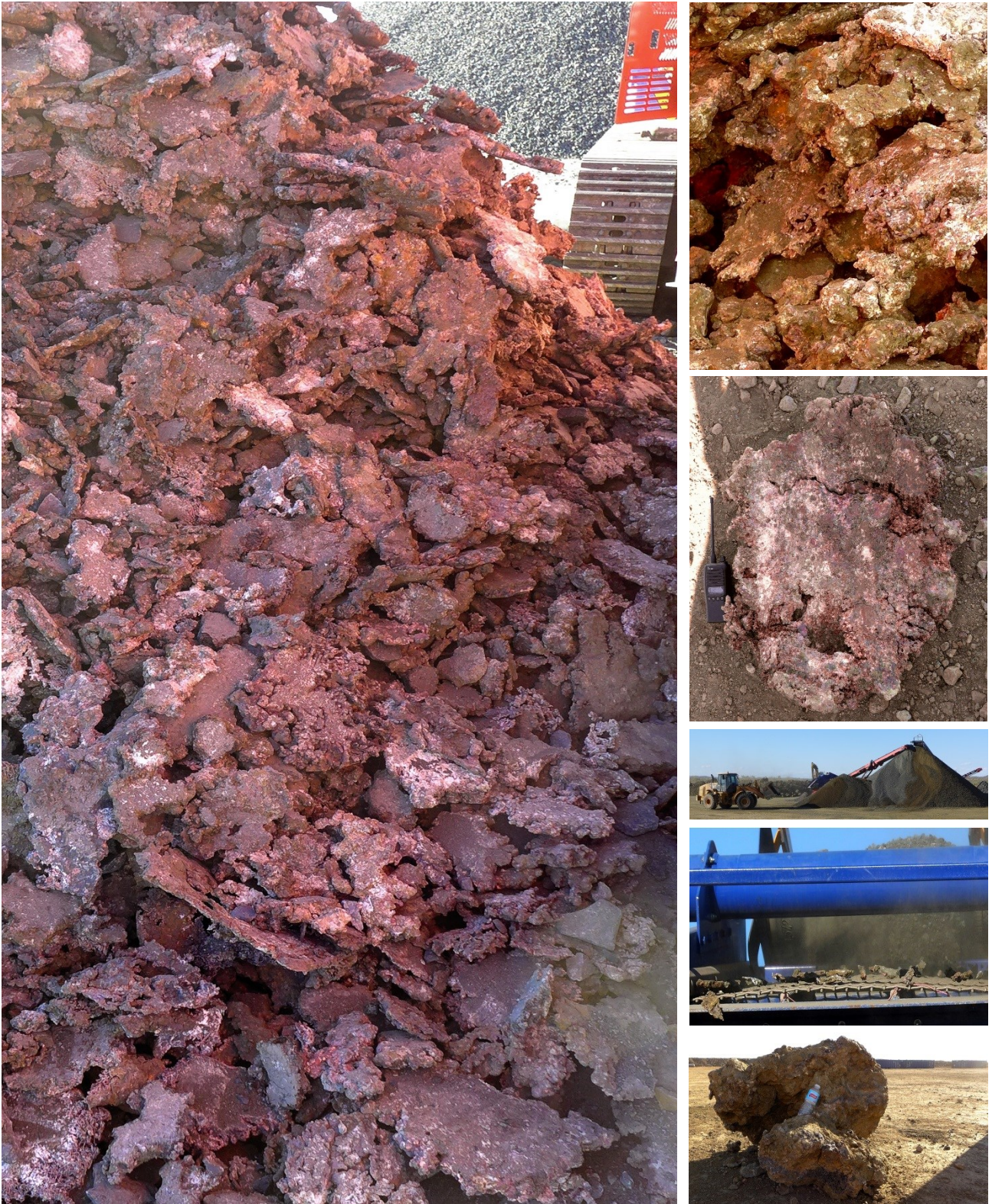
Figure 4: Left; high-grade DSO (+40mm) visually estimated at 90% Cu in this batch, scalped off the crusher screens - predominately native copper (99.65% Cu). Right (top to bottom); close-up of +40mm scraped product; large 60kg copper nugget; -40mm crushed product; containers of +40mm scalped product; up-close detailed image of operating +40mm screens showing flattened native copper being removed; and large native copper nuggets of predominately native copper on the ROM with DSO containers in the background.
