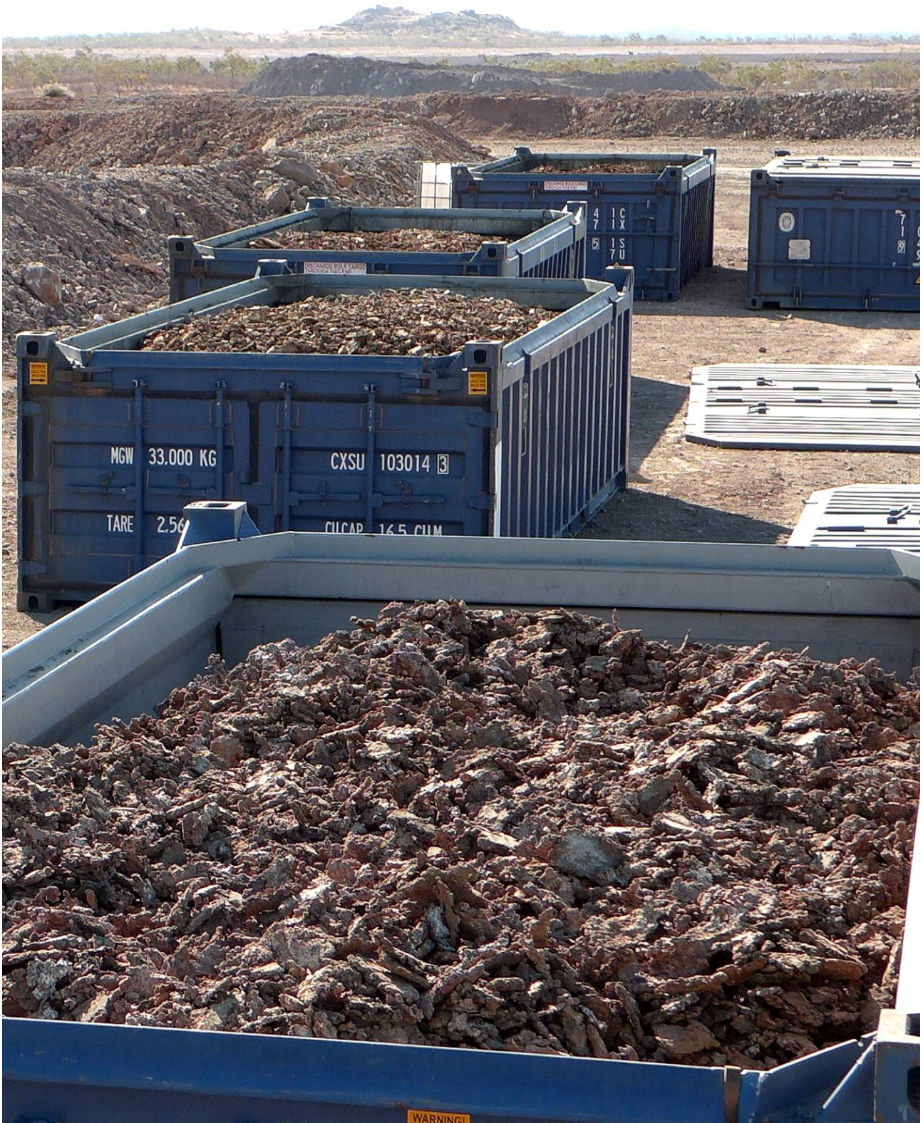
Figure 2: High-grade DSO (+40mm) visually estimated at 80-90% Cu, scalped off the crusher screens and loaded into containers ready for shipment. Each container holds between 22-25 tonnes of predominately native copper (99.65% Cu).
