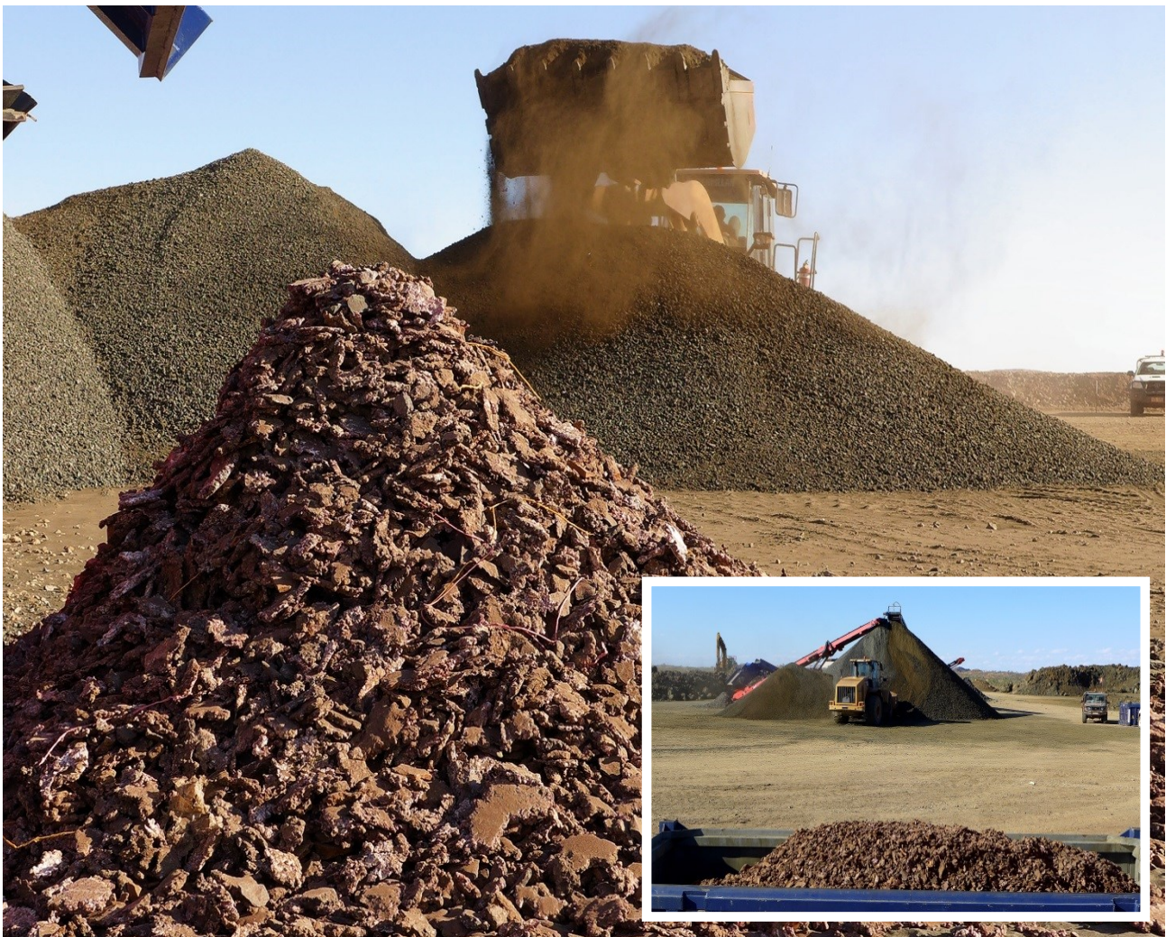
Figure 3: High-grade DSO (+40mm) scalped off the crusher screens. Predominately native copper (99.65% Cu). Inset; crushed product under the -40mm conveyors and +40mm scalped native copper DSO product in containers in foreground.
