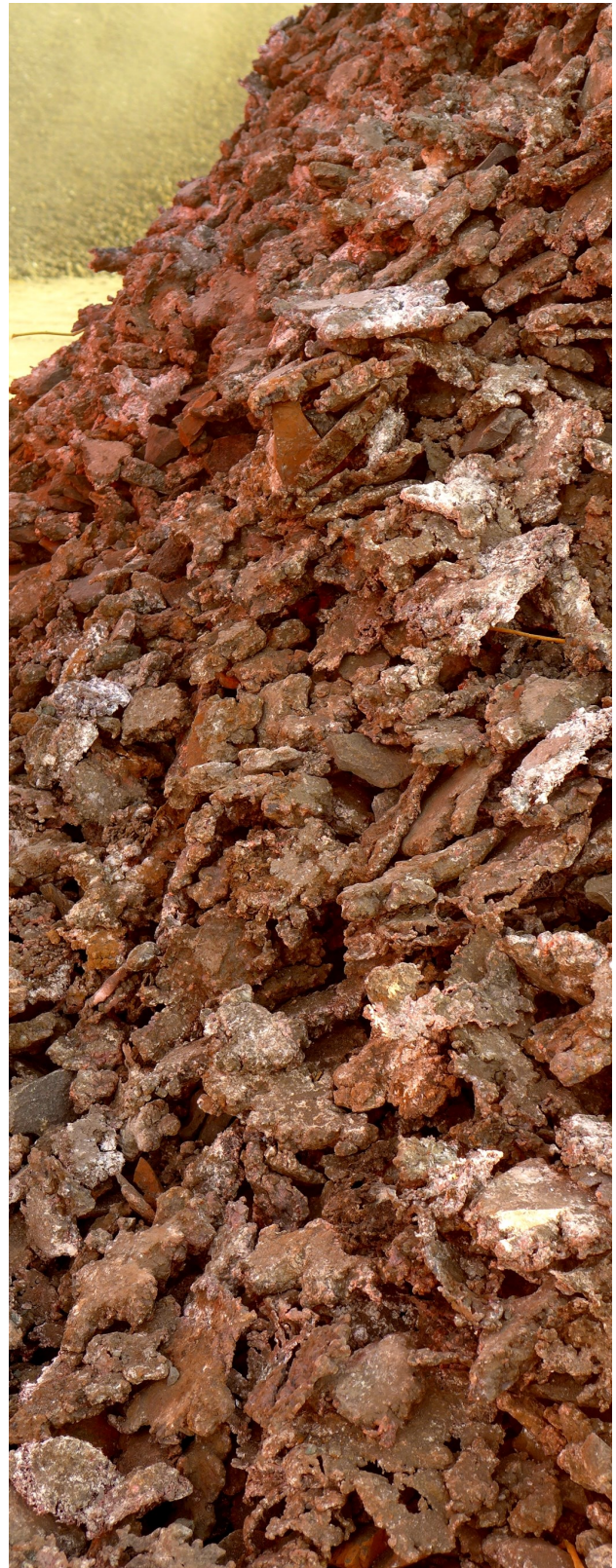
Figure 5: High-grade DSO (+40mm) scalped off the crusher screens, estimated at 90% Cu in this batch.
