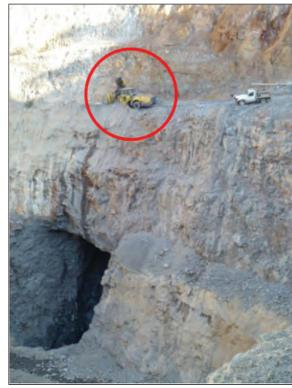
Figure 7-9: Underground production drill, drilling 490 cut off slot from pit ramp
