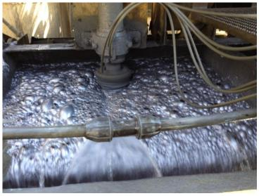
Photo 12 - Flotation Cells
