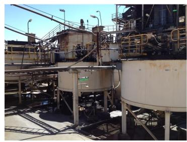
**Photo 14 – Thickeners and Filter Press**
