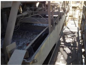
Photo 11 - Flotation Cells
