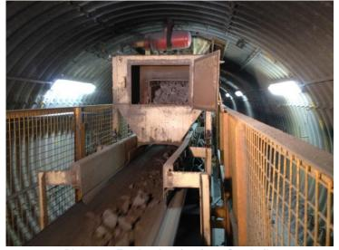
Photo 4 – Feeder drawing from Stockpile
