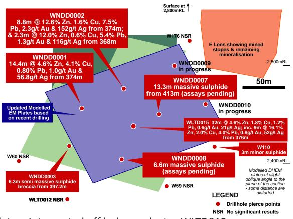
2012 DHEM Plate – Interpreted off hole conductor WLTD012
