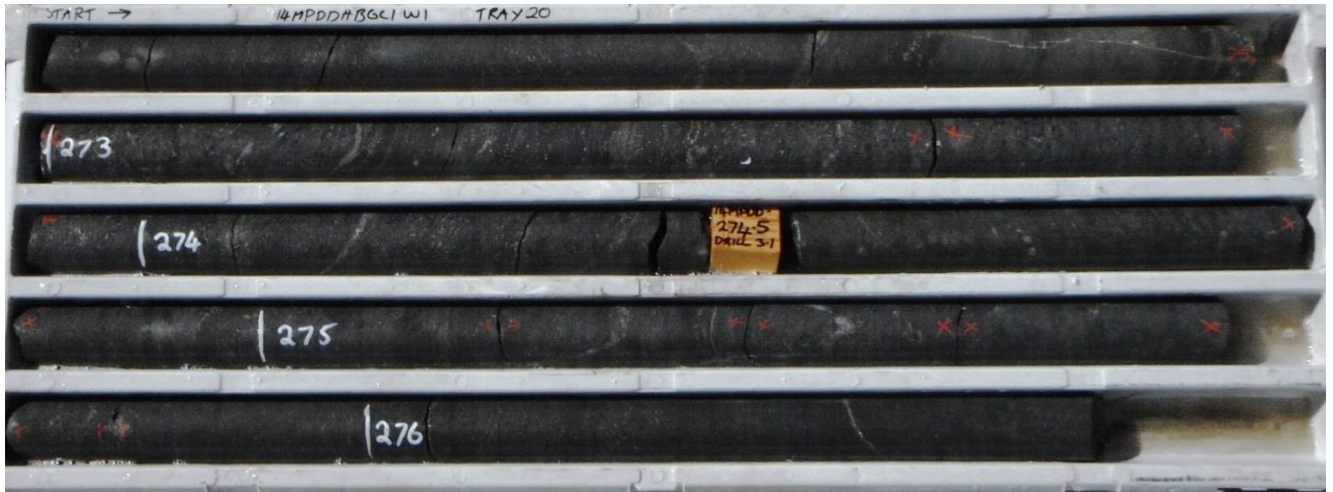
Figure 3. Core tray #20 from 14MPDDHBGC1W1 from 272.1 to 276.7m, showing typical competent dark grey graphitic silica-pyrite core comprising the material in composite “BGC1 HG”.
