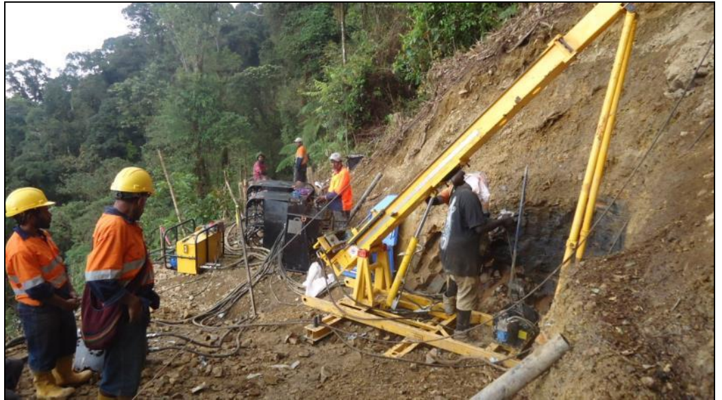
Photo 1. The CSD500 drill rig being set up on pad 1.
