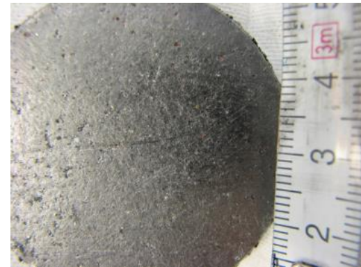
Graphite foil produced from Kibaran large flake graphite
