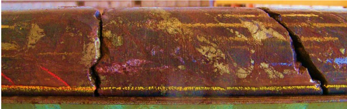
Figure 1 – High grade (+6% Cu) primary sulphide mineralisation intersected by BBDD0004
