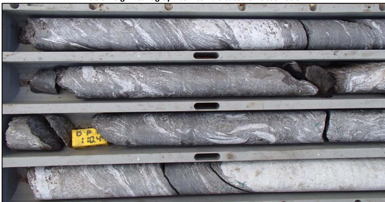
Figure 2. Photo of graphitic drill core from Montepuez Central Project MN0002D, 110m, graphitic shear zone with 10-20% graphite.
