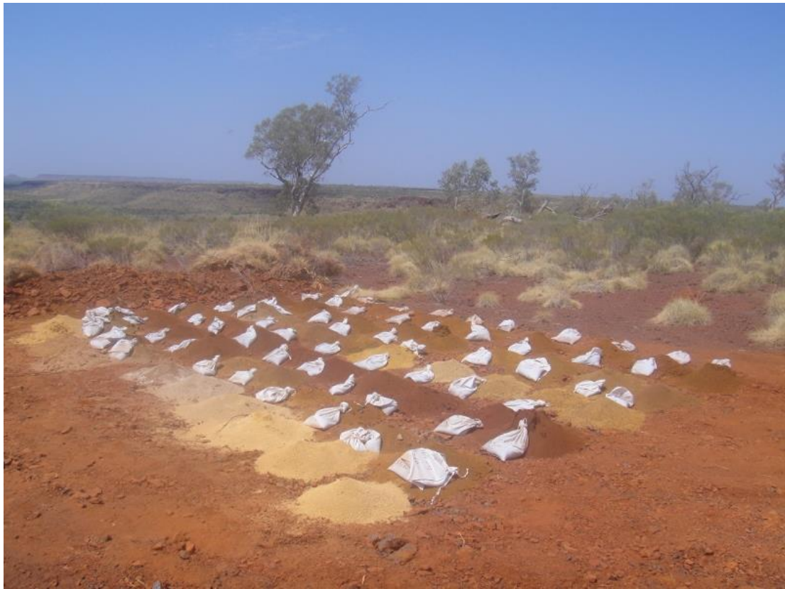
Fig 2. RC drill samples (1m intervals) showing the darker red pisolitic iron-stone upper zone (farthest 2 rows), a lighter coloured shaley interval (1 row) and a darker red lower zone pisolitic iron-stone (1.5 rows) overlying the light-coloured Proterozoic basement (in foreground).
