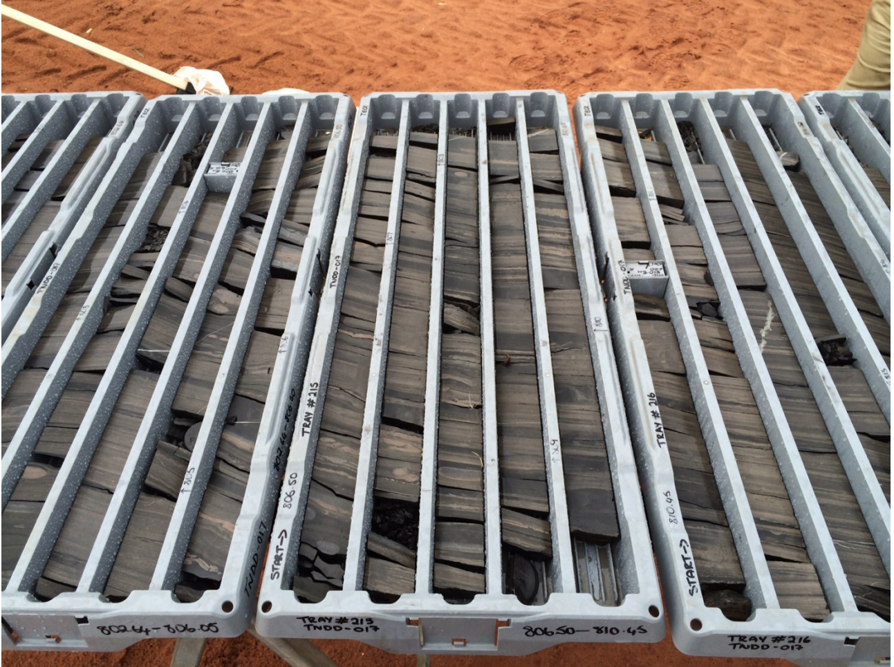
Figure 3: High grade stratiform sulphide mineralisation in drill core from hole TNDD017, 802 – 815m
