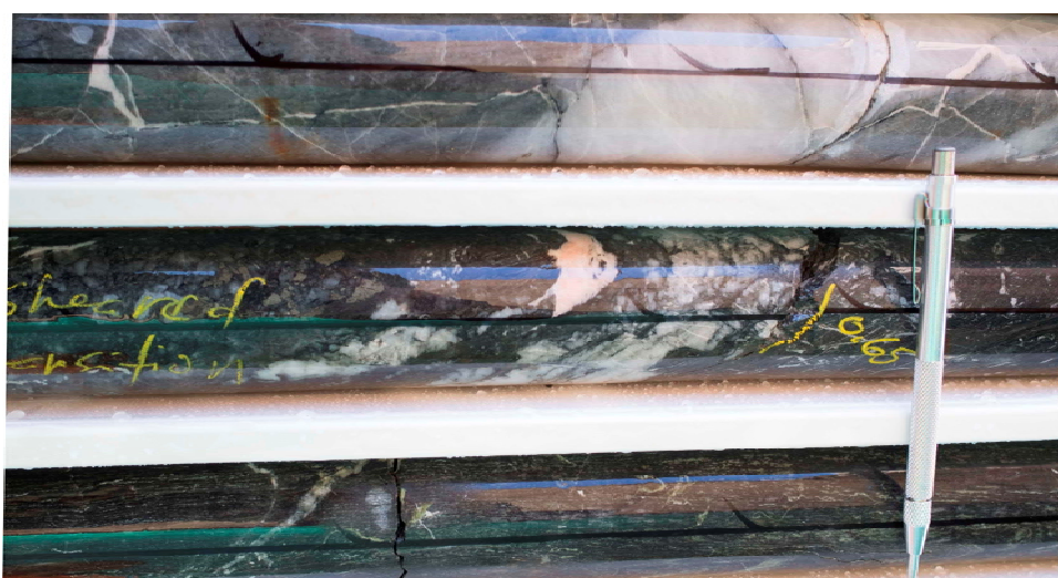
Figure 2: Gruyere drill core from diamond hole 14GYDD0061- approximately 750 metres down hole. Sheared and brecciated quartz veins and strongly altered tonalite (top of photo) proximal to a strongly deformed mafic intrusive (bottom of photo).
