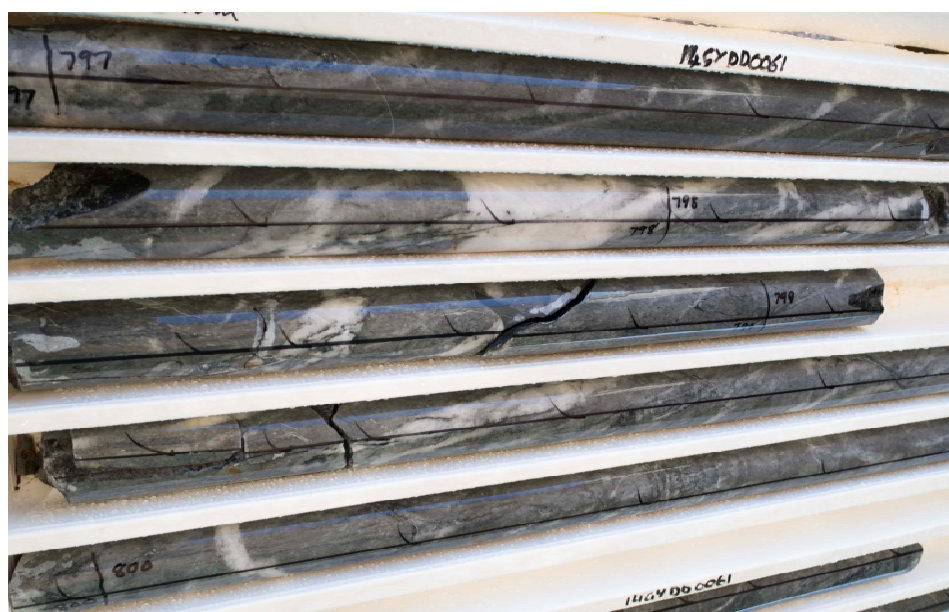
Figure 3: Gruyere drill core from diamond hole 14GYDD0061, 797 metres to 801 metres. Strongly altered tonalite resembles mineralisation within the Northern High-Grade domain in the main part of the Gruyere Resource
