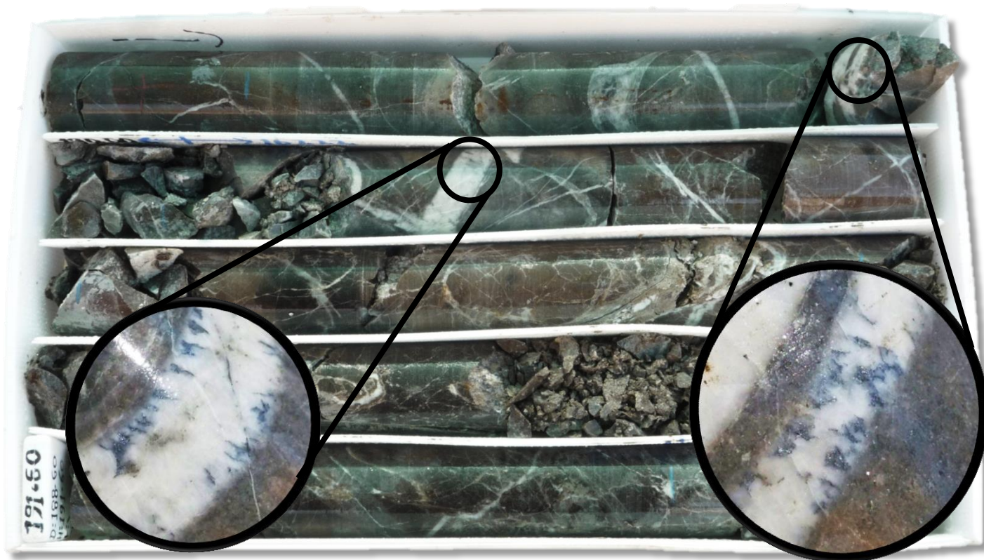
Figure 3 – Core from IE-JDD-003 from 189.35 m to 192.15 m showing typical stockworking and potassic altered quartz micro-diorite porphyry with magnifications showing molybdenite (grey coloured molybdenum sulphide mineral) occurring within the quartz stockworking.
