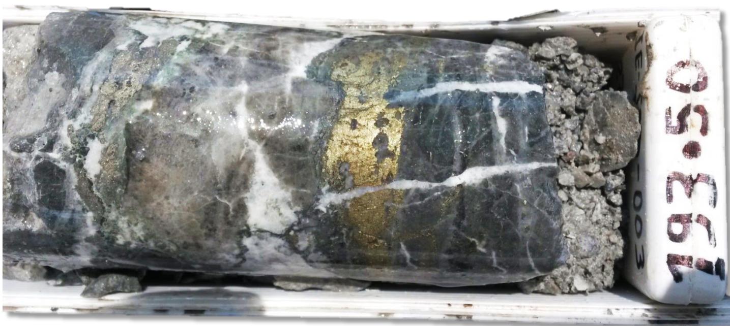
Figure 2 – Copper mineralisation observed as chalcopyrite vein in intensely stockworked and potassic altered quartz micro-diorite porphyry at 193.5m in IE-JDD-003.
