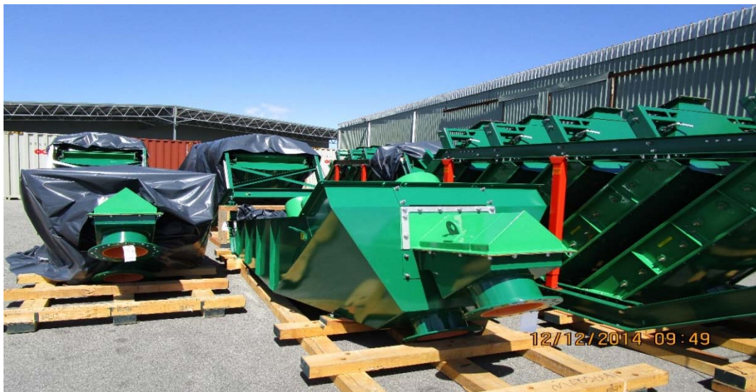
Derrick screens in Perth prior to transport to Windimurra (now at site)
