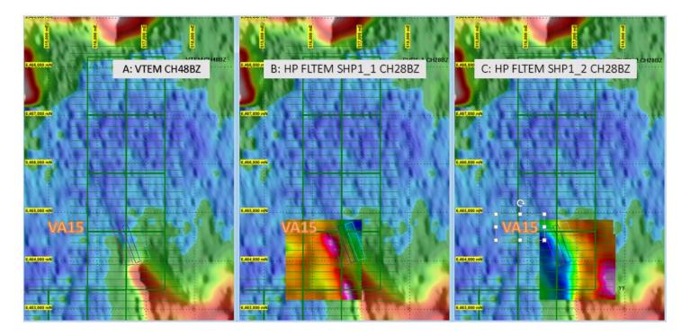
Figure 2: Comparison between VTEM and Late Channel HP FLTEM images from SHP1\_1 and SHP1\_2
