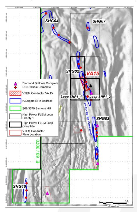
Figure 1: EM Survey Location on aeromagnetic image
