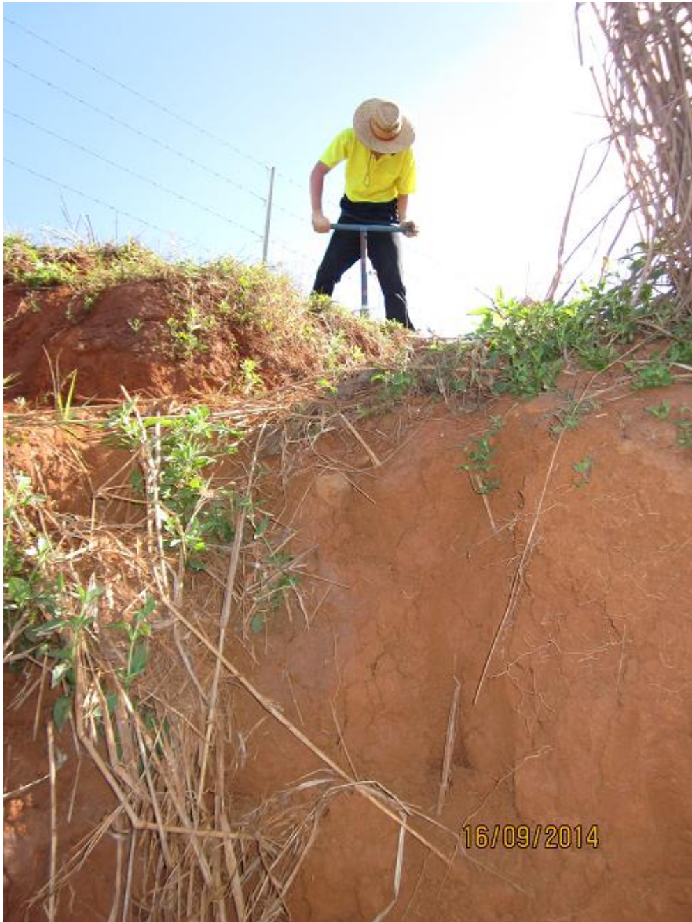
Hand auger surface drilling profiles bauxite at South Johnstone Project
