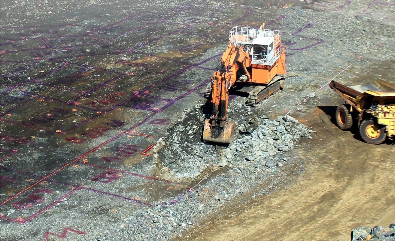
Figure 1: The orebody is marked up on the pit floor by geologists who detail the location and extent of the ore type and copper grades for mining. To illustrate the value of the Las Minerale high-grade native copper zone being mined; each dump truck load of 30% Cu ore carries an approximate value of ~A$210,000 of copper metal per truck. With a dump-truck being loaded every three minutes, approximately A$1m worth of contained copper metal is being mined from these high-grade zones every 15 minutes. The LM1 Pit is currently accessing just 120m strike of the Las Minerale supergene ore zone which has a total strike length of ~600m, continues pervasively to depths of 180m and is up to 45m wide. The 600m long supergene ore zone occurs within the Las Minerale orebody that contains predominately primary sulphides, is up to 120m wide and remains open at depth below the deepest drill intercepts at ~650m.
