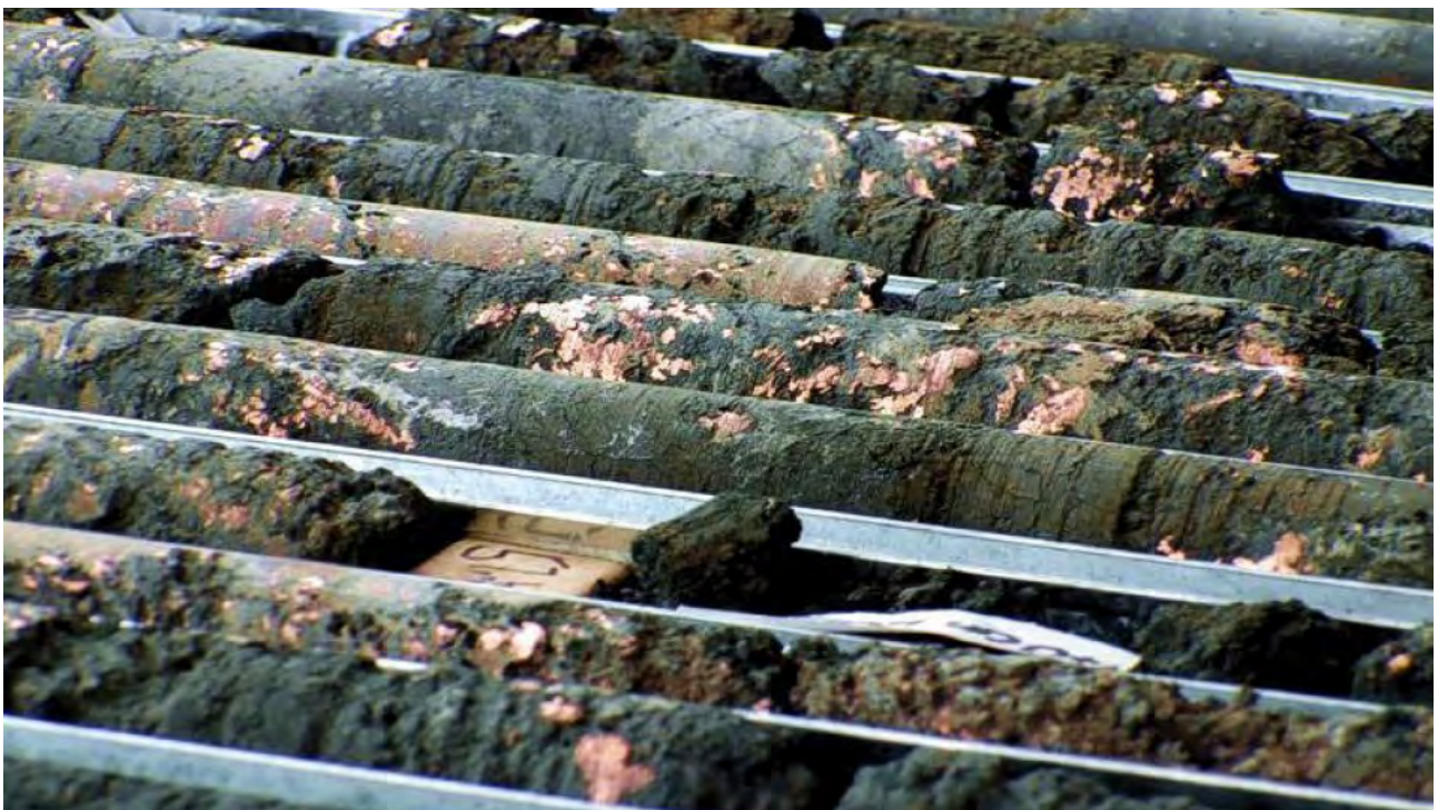
Figure 12: Diamond drill hole LMDH007 - among the first few diamond holes drilled into Las Minerale in the early days of the discovery. Above; copper filings can be seen remaining in the water-return wash-back (above) and drill core from the Bonanza area (intersected in LMDH007) being accessed in the LM1 pit (~51m +/- 5m)
