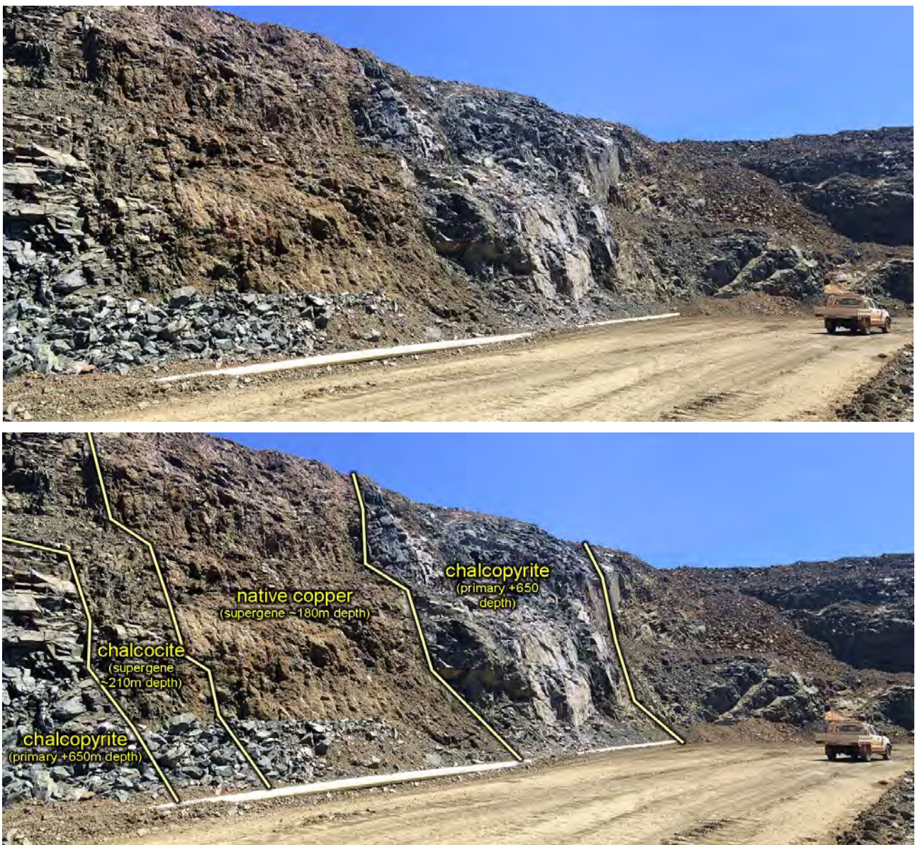
Figure 11: LM1 Pit wall above south haul-road (~45m below surface), showing sub-parallel ore zones that include primary sulphide ore types (chalcopyrite & bornite) and supergene ore types (chalcocite & native copper) in vertically stacked, sub-parallel zones.
