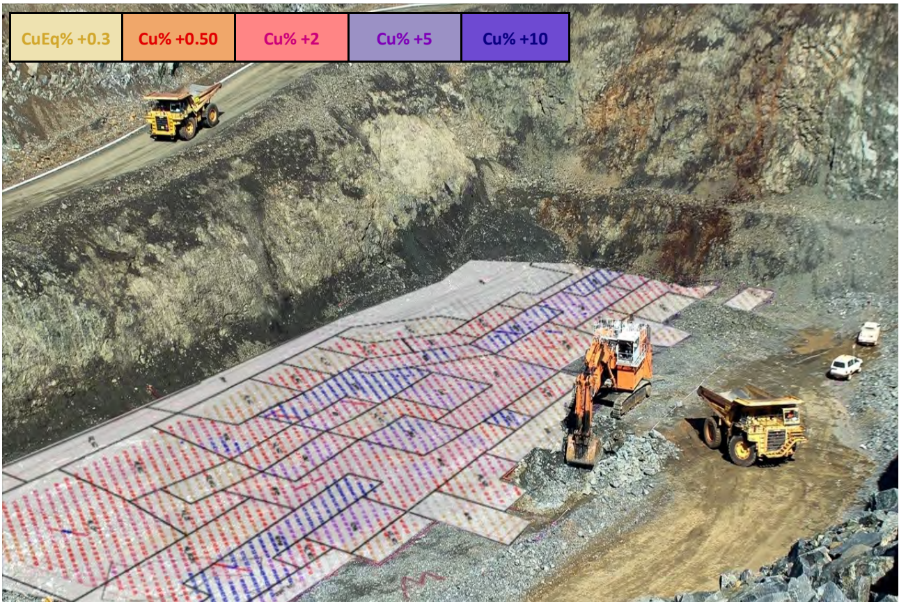
Figure 2: High-resolution ore mark-ups are used in conjunction with careful data control and truck monitoring, to maximise ore control and minimise mining loss and/or mining dilution. The top image shows a close-up of the pit-floor mark-up details including ore boundaries matched to digger capabilities, and the various floor references ore spotters use to guide ore control. The bottom image shows a montage of the pit floor dig-plan (Cu% only) overlaid onto an image of the pit-floor. Dig plans are generated digitally from interpretation of all available data and transferred directly to the pit floor by our surveyors and pit-techs. The ore mark-ups are then used as a guide by the digger operators, with direction and final spot-checking and confirmation by our ore-spotters, to ensure optimised ore management and grade control. Dig plans are generated based on a combination of data including blast-hole sampling and analysis, pit-floor mapping, resource block model estimates and localised results of resource and metallurgical drilling and assay.
