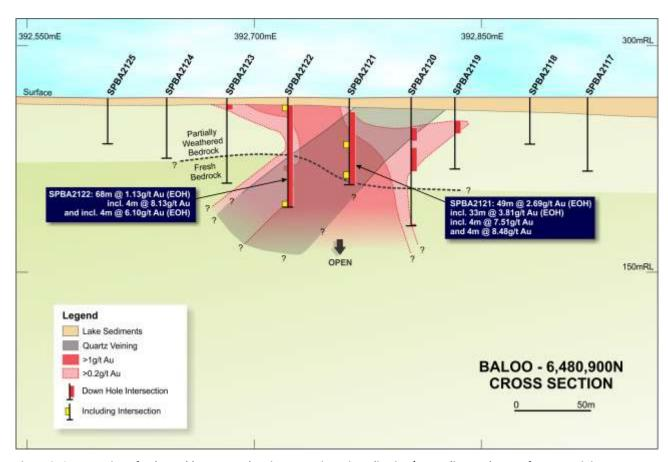
Figure 2. Cross section of Baloo gold prospect showing extensive mineralization/anomalism and zone of quartz veining.
