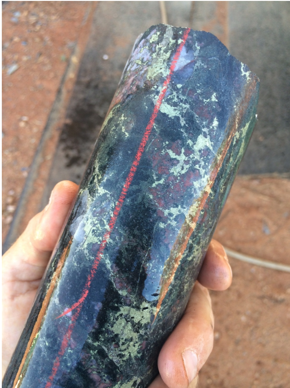
Figure 11: Diamond drill core from hole BYD001. The light yellow mineral is chalcopyrite (copper sulphide), while the red-brown mineral is hematite (which is an alteration mineral associated with copper mineralisation), and the dark green mineral is probably chlorite and/or amphibolite. The white mineral near the holder's thumb is quartz.
