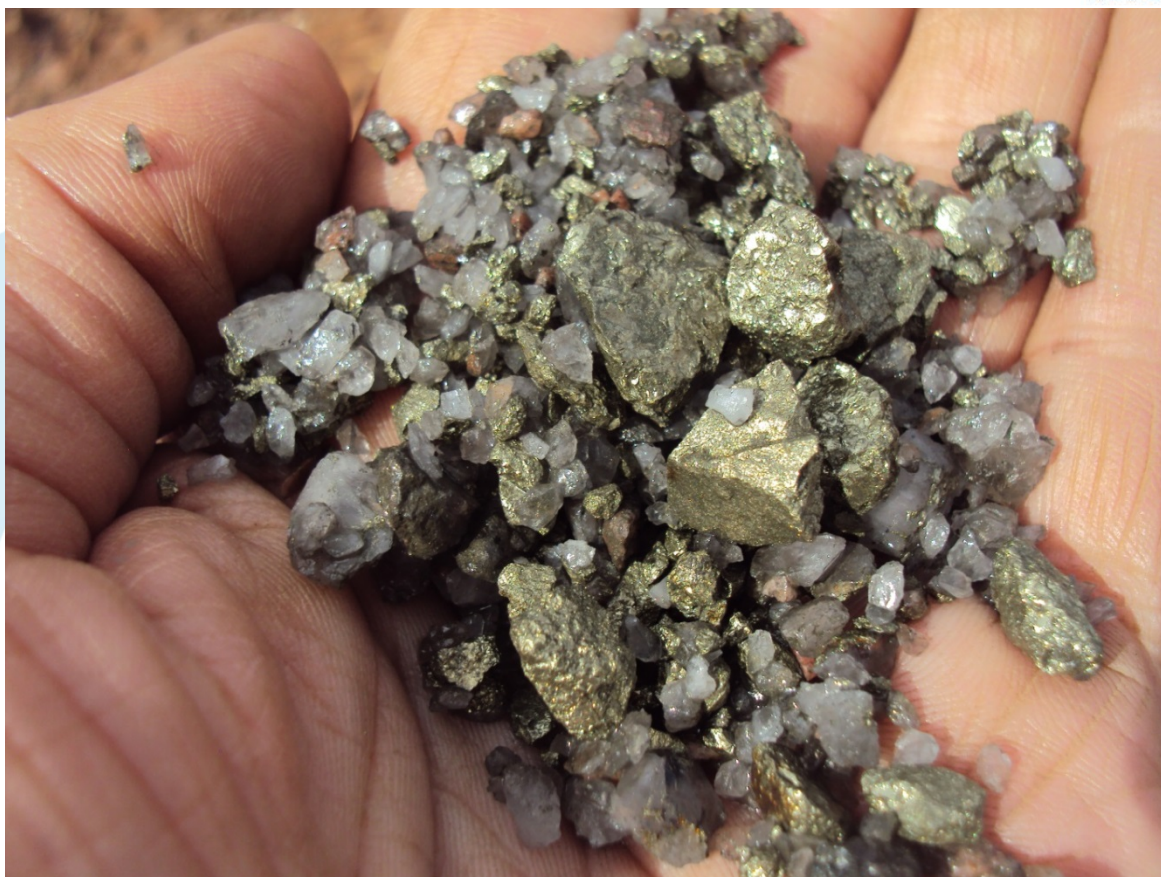
Figure 9: RC chips from hole BYRC018 – the brassy yellow mineral in abundance is the copper sulphide, chalcopyrite
