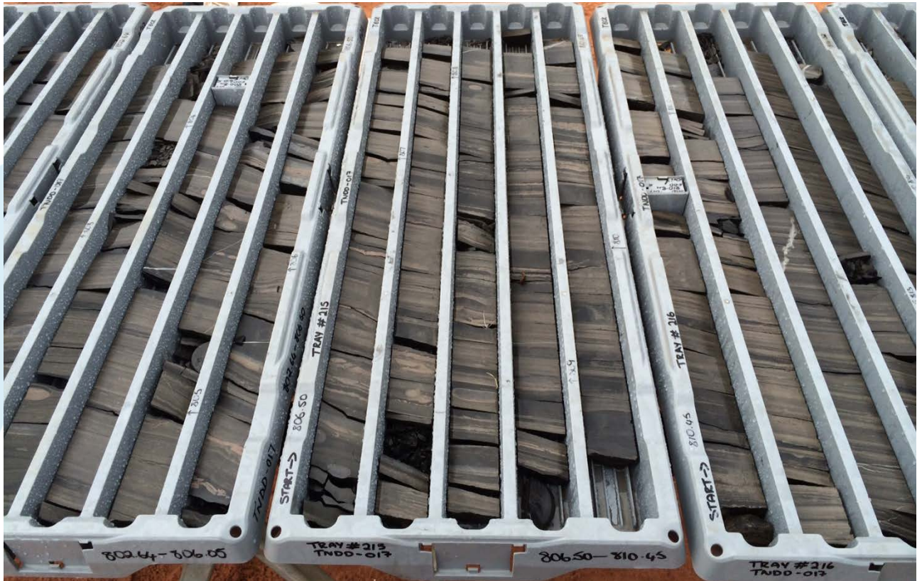
Figure 14: High grade stratiform sulphide mineralisation in drill core from hole TNDD017, 802 – 815m
