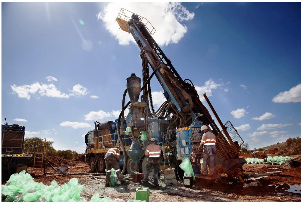
Figure 4: Racetrack Diamond Drilling
