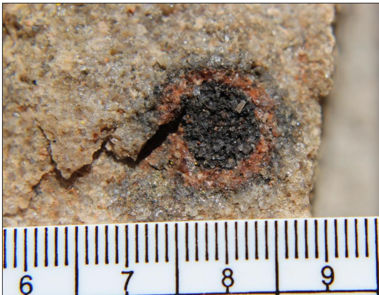
Figure 7 – Uranium-bearing pyrite-rich sphere in sandstone containing smoky quartz, rimmed by orange, radiation-damaged potassium feldspar, Walbiri Deposit hole WPD7 (193.1m).
