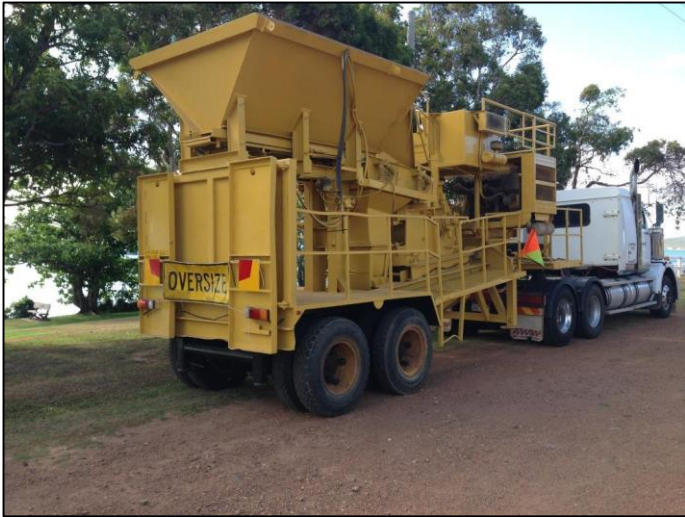
Picture 14: Primary crusher being transported to site.
