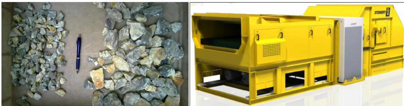
Pictures 6 and 7: The shear material sized for sorting and a typical Steinert X-ray Sorting System (XSS) machine.
