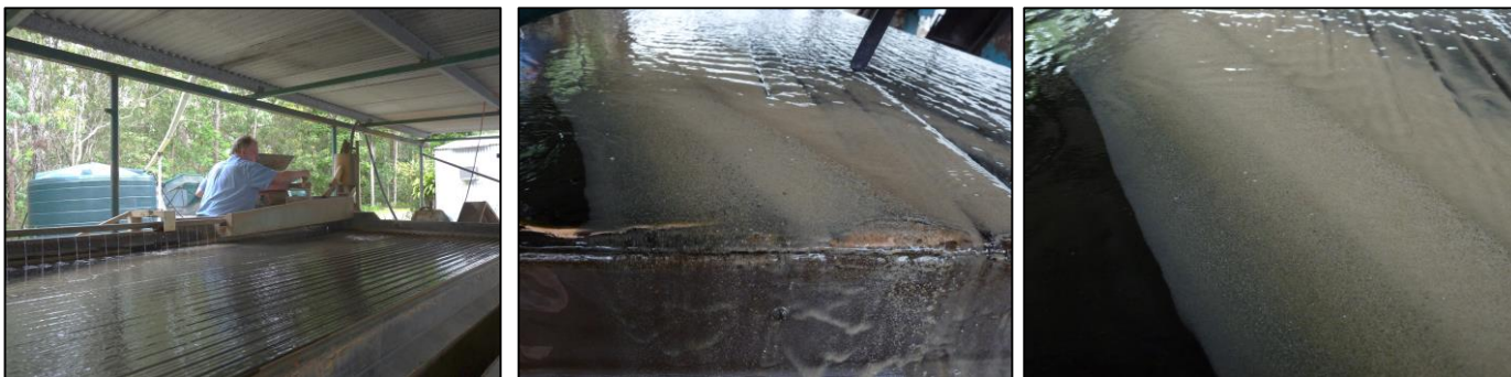
Pictures 8, 9 and 10: Gravity table trial with distinct separation of high and medium grade concentrates and waste.
