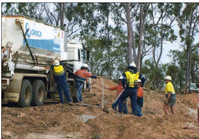
Pictures 1 and 2: Prior operations at Norton Gold Mine charging blast holes and mining with excavator and trucks.
