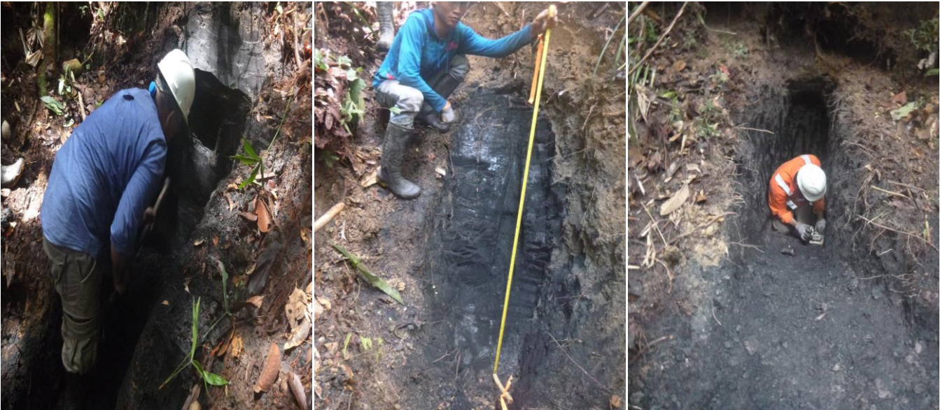
Photo 1: Channel Sampling Coal Outcrops from the Proposed Open Pit –2 in BBM East Block
