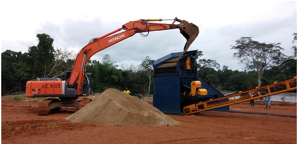
Photograph 3 – Feeding of tailings into the Feed Bin during first phase commissioning of the DMS plant.
