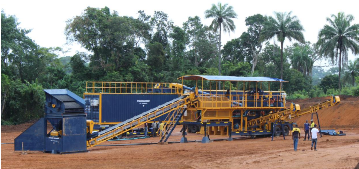
Photograph 1 – Assembly of DMS plant on-site at the Baoma Project, Sierra Leone
