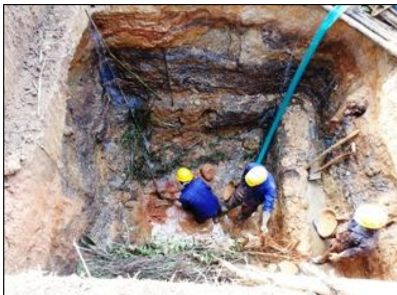
Figure 6. Basal gravel intercept from a Makombo Target maxi-exploration pit (at left). Note detail of organic debris at base of palaeo-channel system, and water ingress (at right), suggesting a stranded palaeo-channel, deposited some distance from the Modern Sewa River.
