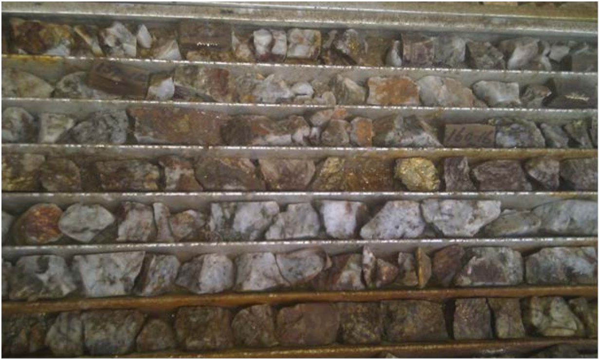
Figure: Mineralised zone of massive quartz within historic Geopeko drillhole DDH4, with patchy sericite and massive or blebby chalcopyrite. Coarse molybdenite is also present. Interval from 158-164m returned 2.64 % Cu, 908 ppm Mo and 9 ppm Ag. (CR4994, Report on Griselda-Discoverer 28, Geopeko Ltd, May 1974).
