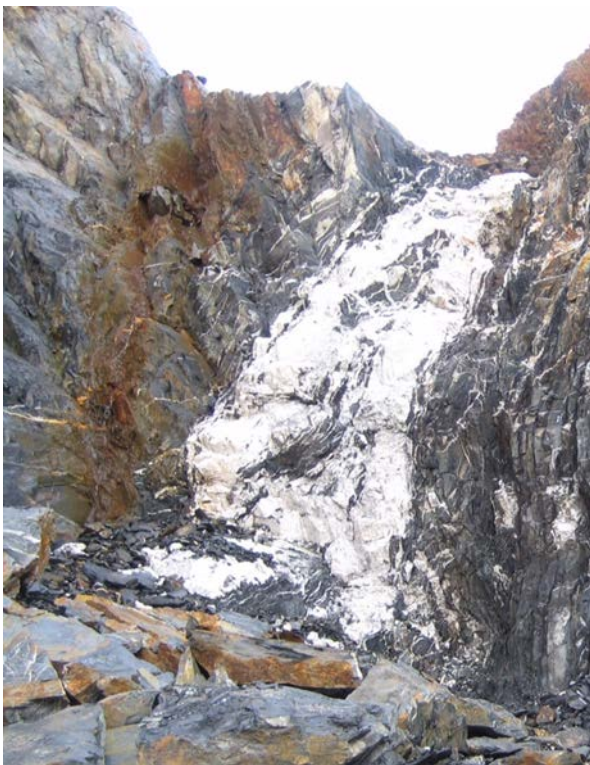
Photograph; Main lode mineralised quartz vein (Vein width of approximately 1 m). Veins are sub-parallel to the beddings. Figure; wireframe of main lode structural zone, drill holes and current pit surface and pre-mining land surface.
