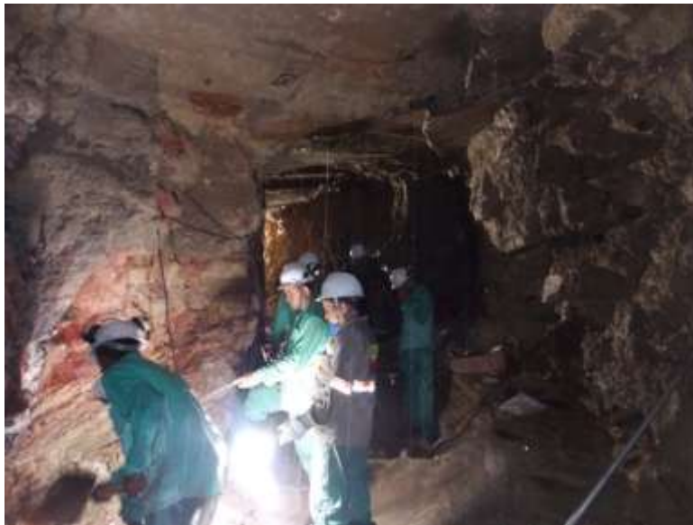
Figure 3. Cleaning the face of the exploration decline ahead of sampling.
