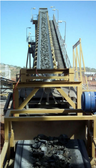
Figure 05: Conveying ore from the Primary Jaw Crusher to the screen above No 1 Rolls Crusher
