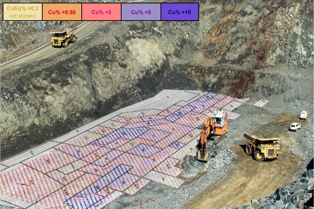
Figure 22: High-resolution ore mark-ups are used in conjunction with careful data control and truck monitoring, to maximise ore control and minimise mining loss and/or mining dilution. The top image shows a close-up of the pit-floor mark-up details including ore boundaries matched to digger capabilities, and the various floor references ore spotters use to guide ore control. The bottom image shows a montage of the pit floor dig-plan (Cu% only) overlaid onto an image of the pit-floor. Dig plans are generated digitally from interpretation of all available data and transferred directly to the pit floor by our surveyors and pit-techs. The ore mark-ups are then used as a guide by the digger operators, with direction and final spot-checking and confirmation by our ore-spotters, to ensure optimised ore management and grade control. Dig plans are generated based on a combination of data including blast-hole sampling and analysis, pit-floor mapping, resource block model estimates and localised results of resource and metallurgical drilling and assay.
