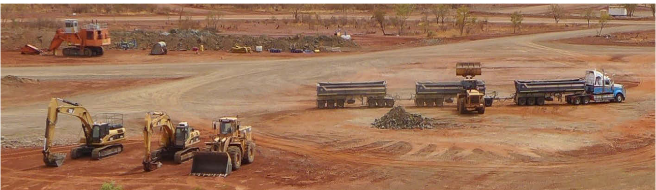
Figure 38: Final truck loads of ore loaded onto haul-trucks. A total of 22,000 tonnes of primary ore was delivered to EHM.
