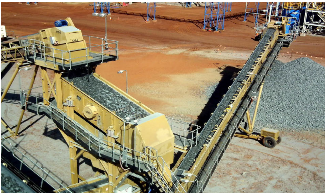
Figure 03: Scalping screen used for removal of the coarse (+40mm) native copper
