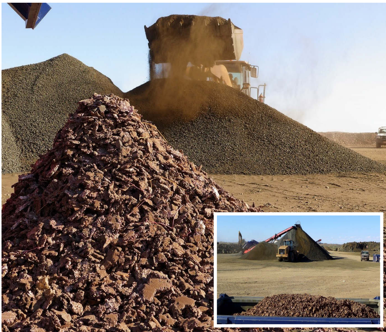
Figure 13: High-grade DSO (+40mm) scalped off the crusher screens. Predominately native copper (99.65% Cu). Inset; crushed product under the -40mm conveyors and +40mm scalped native copper DSO product in containers in foreground.
