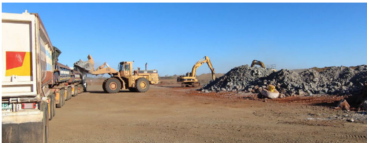
Figure 08: Contractor loading road trains with Rocklands primary ore ready for shipment to EHM processing plant
