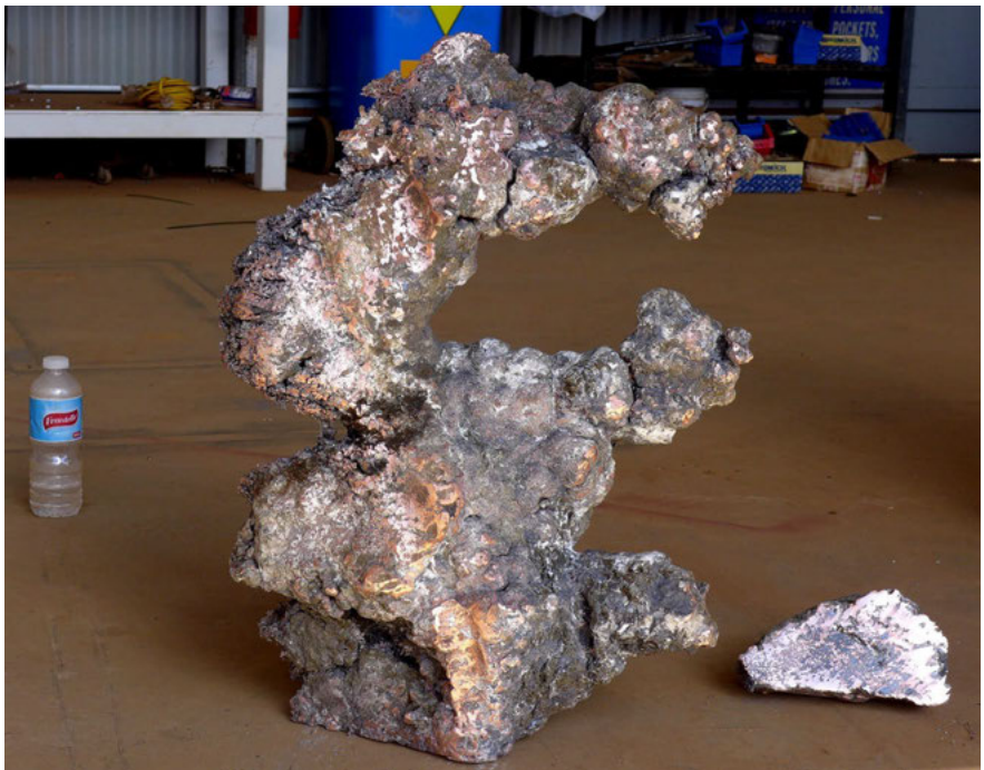
Figure 06 (right); large predominately native copper mass weighing ~130kg, with marks from the mobile jaw crusher imprinted onto its surface.
