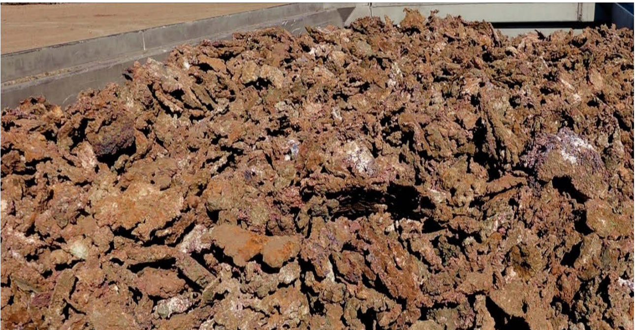
Figure 10: Container full of DSO straight from the crusher screens estimated 85-95% Cu, (+40mm -110mm)
