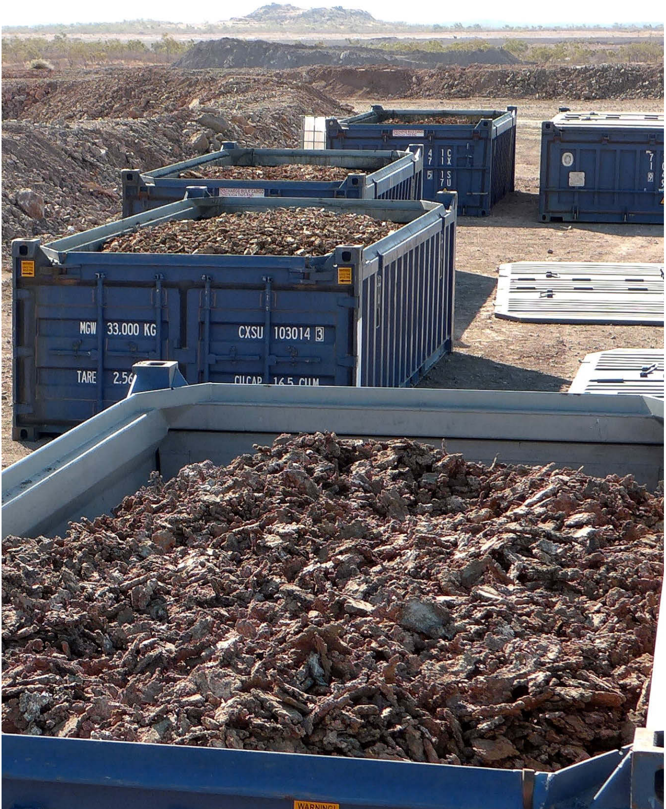
Figure 11: High-grade DSO (+40mm) visually estimated at 80-90% Cu, scalped off the crusher screens and loaded into containers ready for shipment. Each container holds between 22-25 tonnes of predominately native copper (99.65% Cu).
