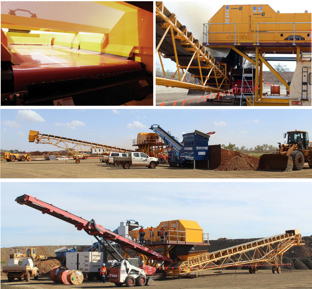
Figure 39: View inside separating conveyor (top left), point of separation of product/waste (top right), Ore-sorter circuit (middle) and bump-testing and setting optimisation (bottom)
