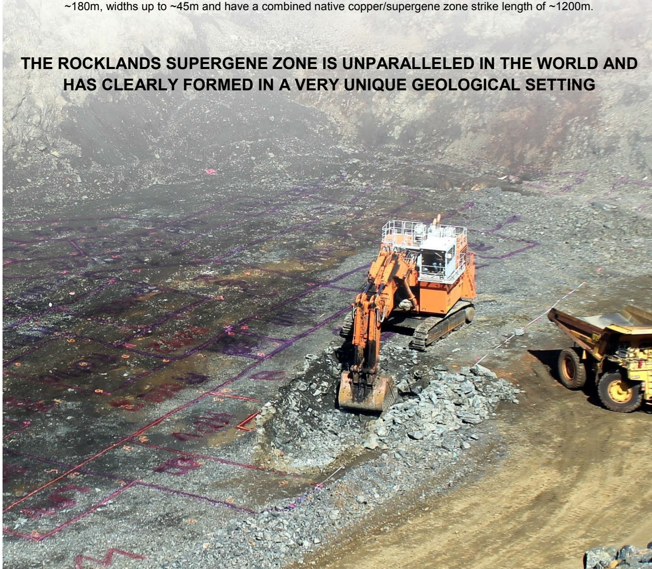
Figure 21: The orebody is marked up on the pit floor by geologists who detail the location and extent of the ore type and copper grades for mining. To illustrate the value of the Las Minerale high-grade native copper zone being mined; each dump truck load of 30% Cu ore carries an approximate value of ~A$210,000 of copper metal per truck. With a dump-truck being loaded every three minutes, approximately A$1m worth of contained copper metal is being mined from these high-grade zones every 15 minutes. The LM1 Pit is currently accessing just 120m strike of the Las Minerale supergene ore zone which has a total strike length of ~600m, continues pervasively to depths of 180m and is up to 45m wide. The 600m long supergene ore zone occurs within the Las Minerale orebody that contains predominately primary sulphides, is up to 120m wide and remains open at depth below the deepest drill intercepts at ~650m.
