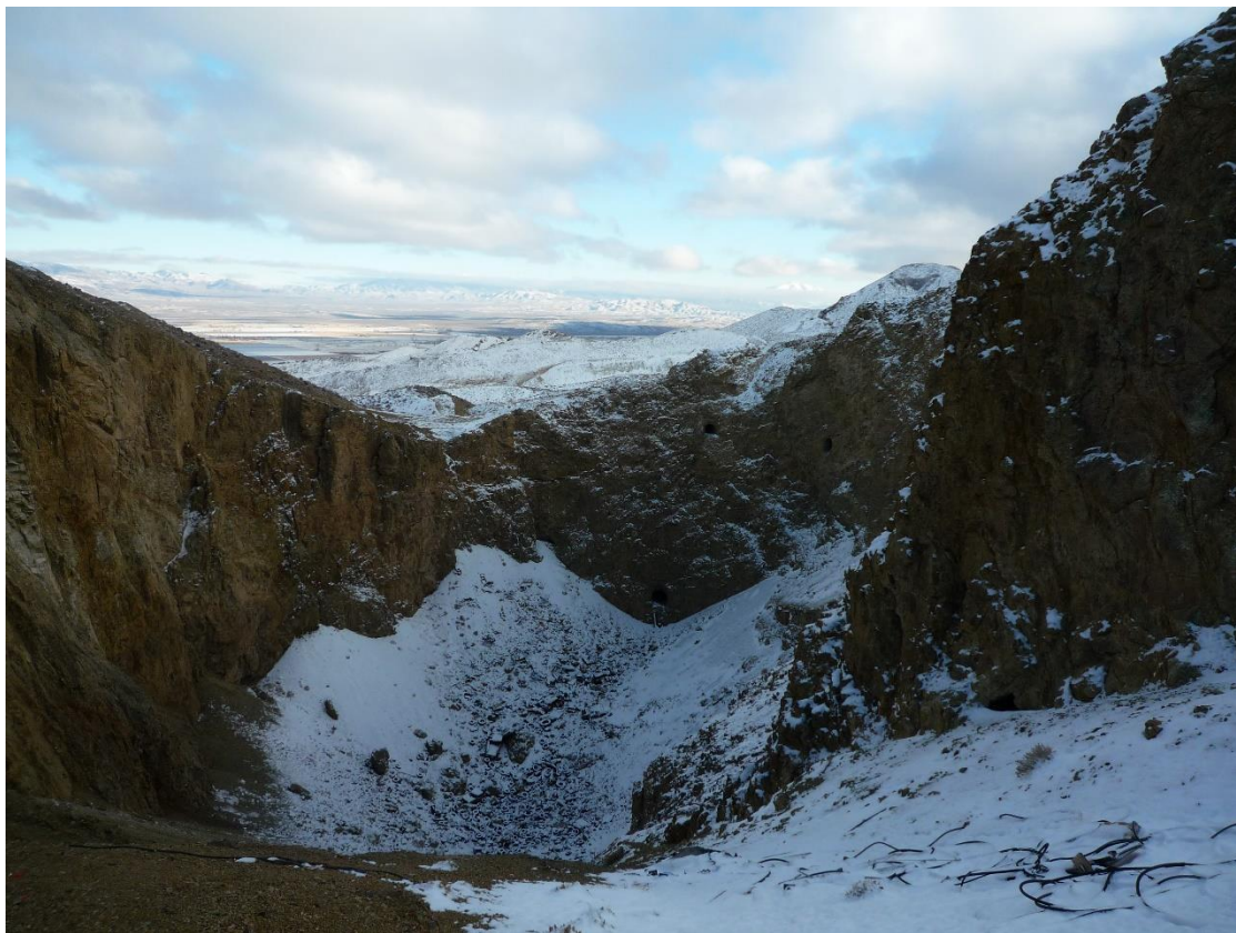
Figure 9: Bluestone copper mine 'glory hole' measuring 150m x 120m x 60m deep with underground development surrounding and below the 'glory hole'.
