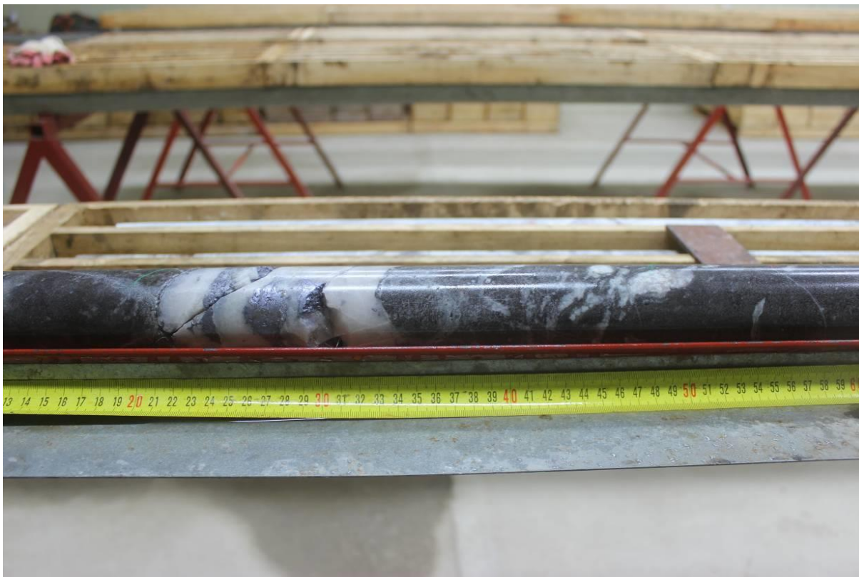
Figure 6: Steeper easterly dipping high grade quartz wolframite (wf) and scheelite (sc) bearing vein 0.18m @ 0.03% Mo & 3.57% W from 321.84m hole DW003_2014.
