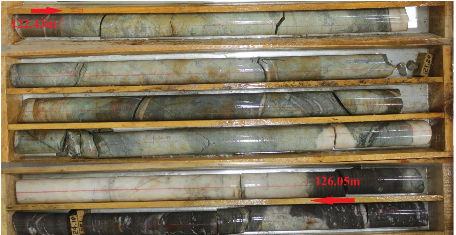
Figure 11: Scheelite mineralisation (blue circles) associated with strong skarn alteration in hole DW005_2014, 3.62m @ 0.02% Mo & 0.05% W from 122.43m (note core blocks out by 3m).
