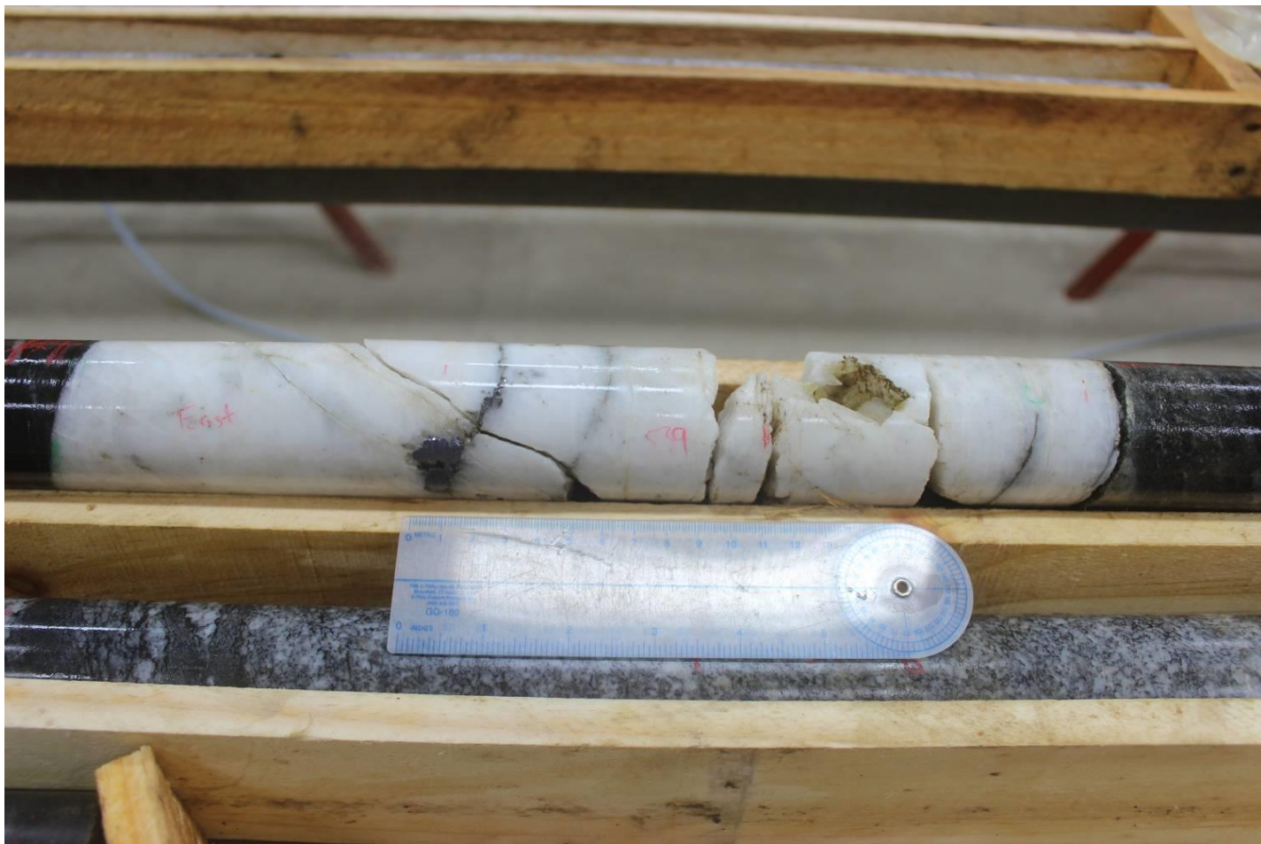
Figure 9: Footwall Mo bearing vein from hole DW009_2014 bucky quartz with coarse nuggetty Molybdenite mineralisation, 0.35m @ 0.13% Mo from 538.76m.
