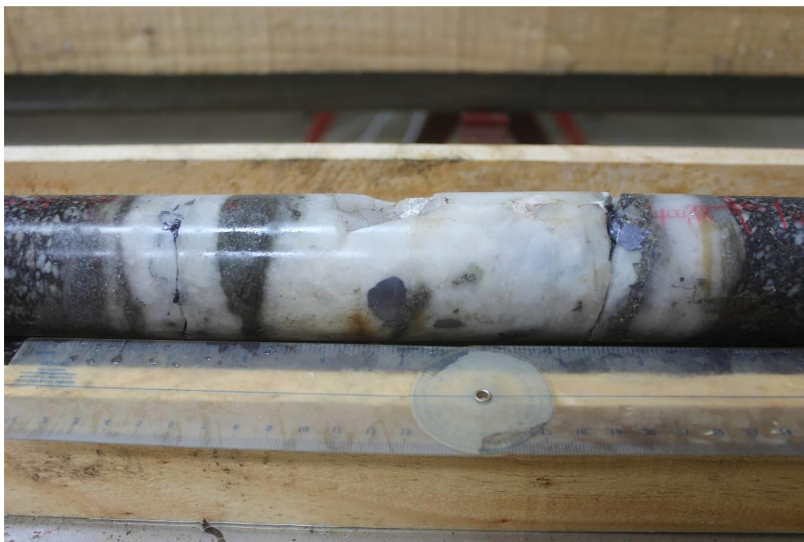
Figure 8: High grade molybdenite bearing quartz vein structure 0.22m @ 4.21% Mo from 400.76m in hole DW001_2014.
