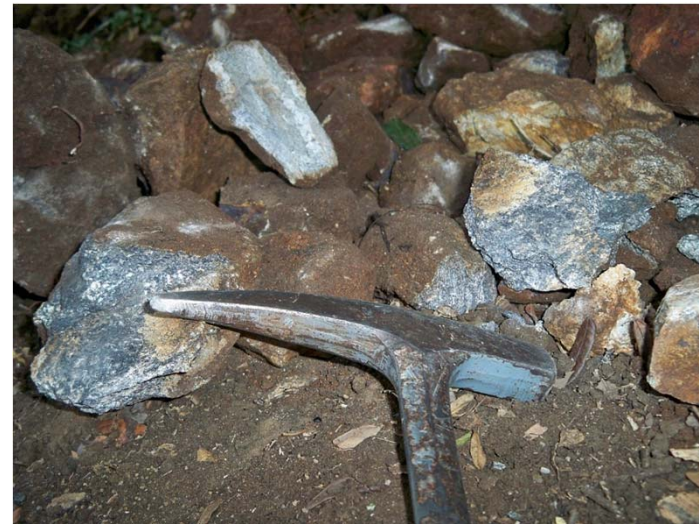
Graphitic schist unearthed via trenching containing 13.7% TGC
