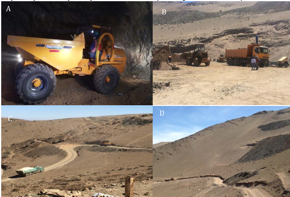
Figure 3- Photos of current activities at San Sebastian – A) 6 tonne underground haulage dump truck underground at San Sebastian B) truck being loaded at San Sebastian with high grade copper material C) trucks departing San Sebastian to the ENAMI plant D) bulldozer preparing access for the 1000 level, note San Sebastian ROM pad above the bulldozer.
