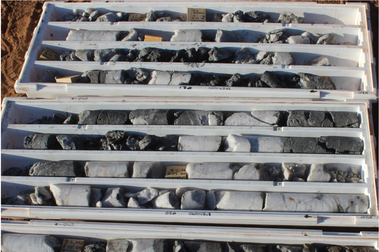
Figure 5. First core from diamond drill hole SPBD0090, showing quartz veins in primary zone.
