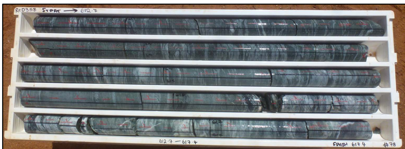
Plate 6 – (612.7 – 617.4m depth) Altered basalt with intermittent minor sulphide bearing quartz veining of various orientations and carbonate alteration.
