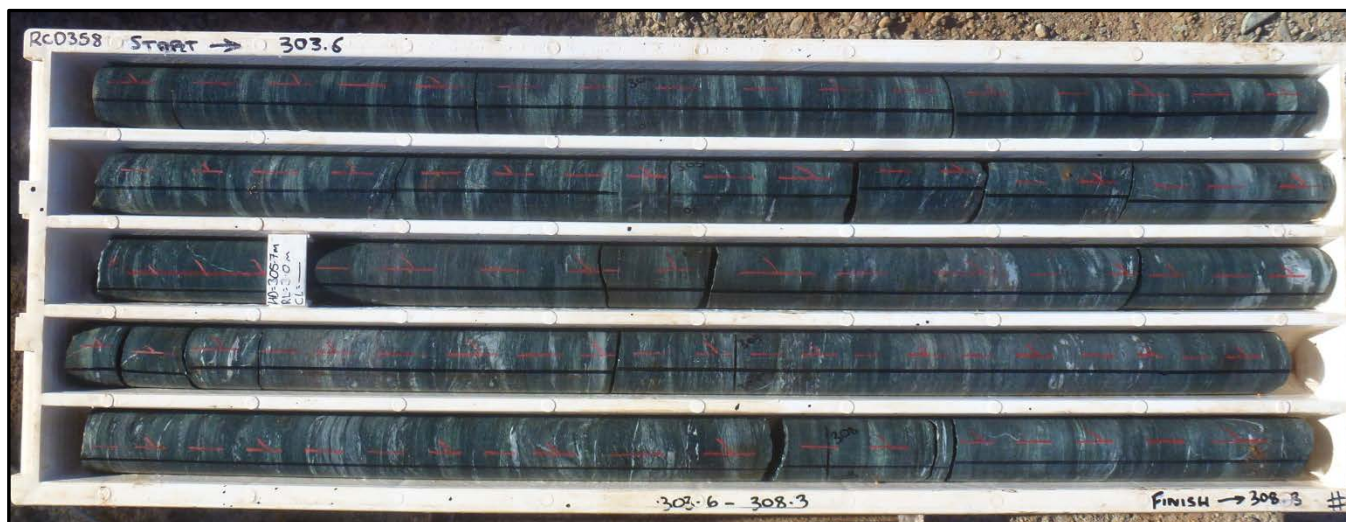
Plate 1 – (303.6 – 308.3m depth) Fine – medium grained metamorphosed porphyritic andesite with minor felsic tuffaceous intervals.
