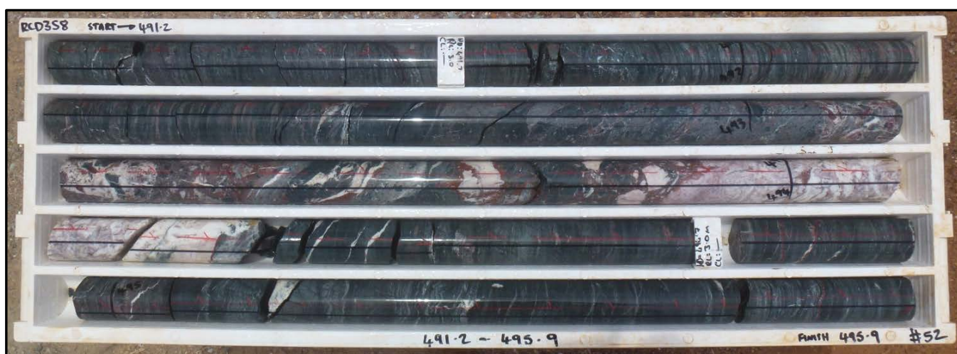
Plate 5 – (491.2 – 495.9m depth) Metamorphosed porphyritic andesite. Strong foliation and chlorite alteration to 492.2m. 492.2 – 494.4m - Contact Zone - Brecciated tuff and basalt clasts within quartz vein with iron rich fluids.
