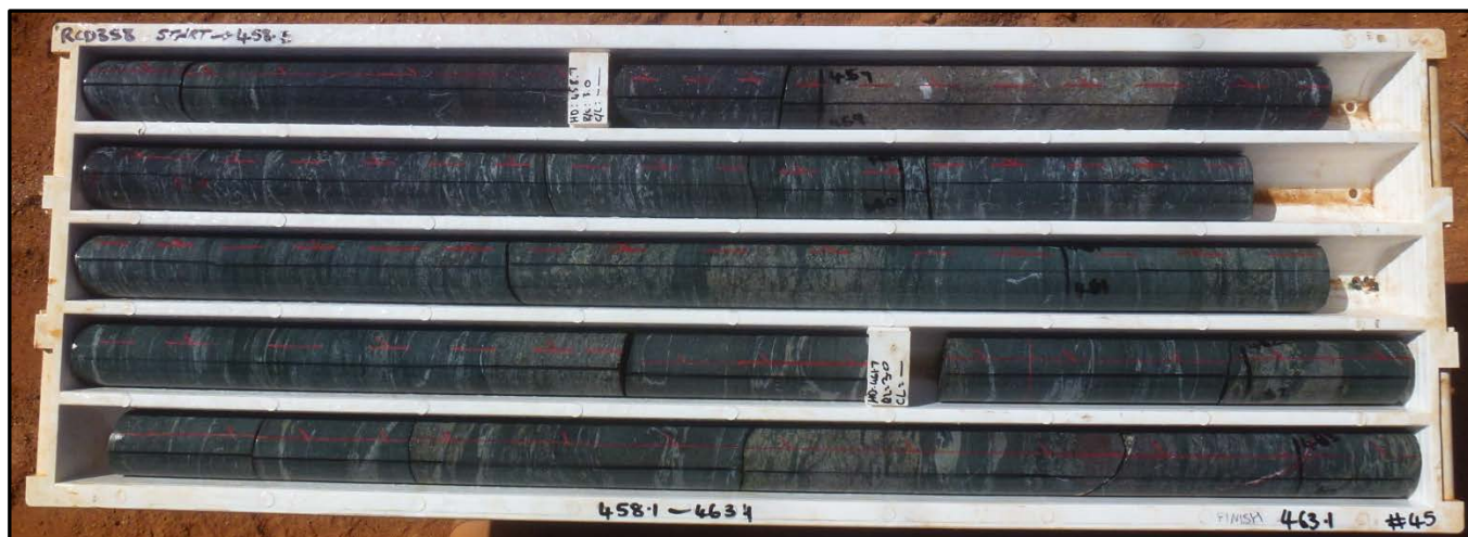
Plate 4 – (458.1 – 463.4m depth) Less altered matrix supported volcanoclastic composed of porphyritic andesite clasts with tuffaceous intervals and some silica and chlorite alteration.
