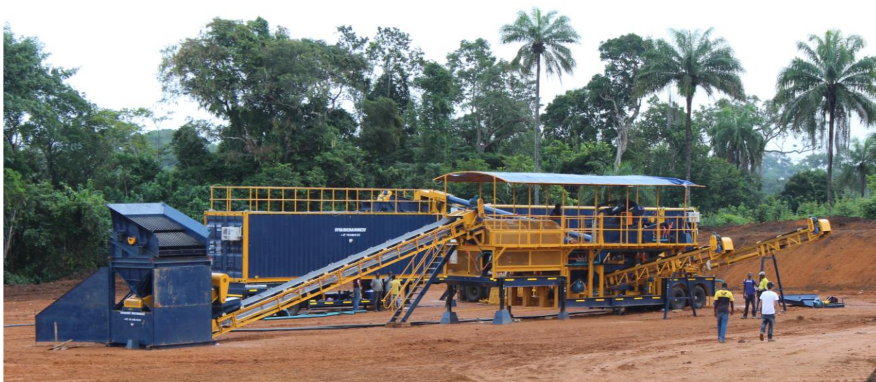
Photograph 5 – Assembly of DMS plant on-site at the Baoma Project, Sierra Leone
