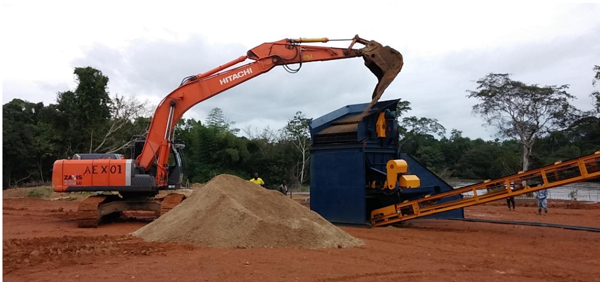
Photograph 7 – Feeding of tailings into the Feed Bin during first phase commissioning of the DMS plant.
