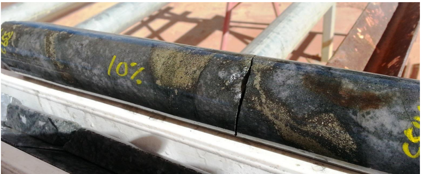
Figure 7: Stringer sulphides (chalcopyrite and pyrite) at 340m downhole in NRD15002. Length of NQ core in photo approximately 0.7 metres.
