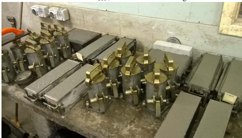
Figure 1 Cylinders of Concrete to be Tested in Australian Trials
