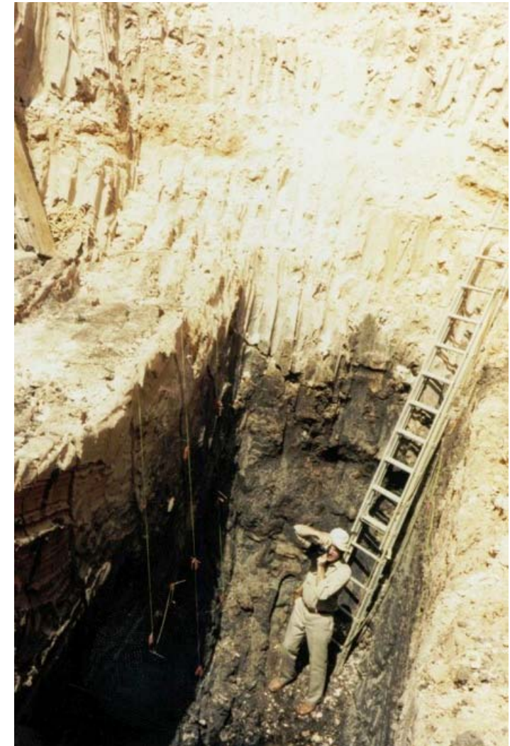
Close-up in test pit showing lignite ore and free dig nature of material
