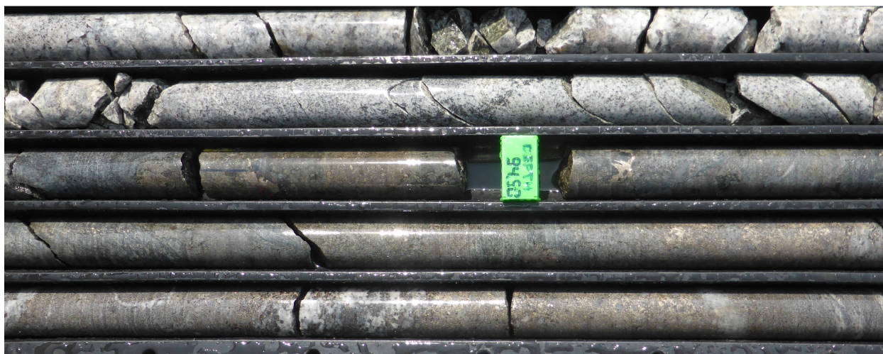
Figure 1 AKD004 showing brecciated zone below granite dyke at 94.3 to 96.4m
