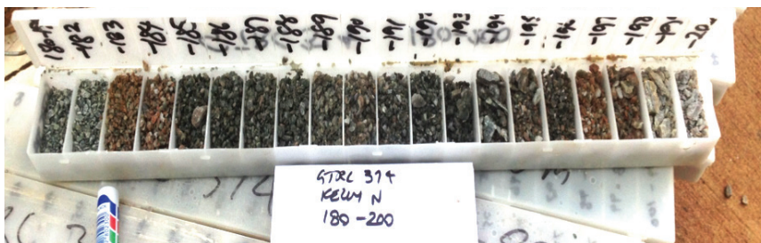
GTRC374 Chip Tray RC Samples 180 - 200m. A result of 2m @ 7.4 g/t Au from 183m was returned.
