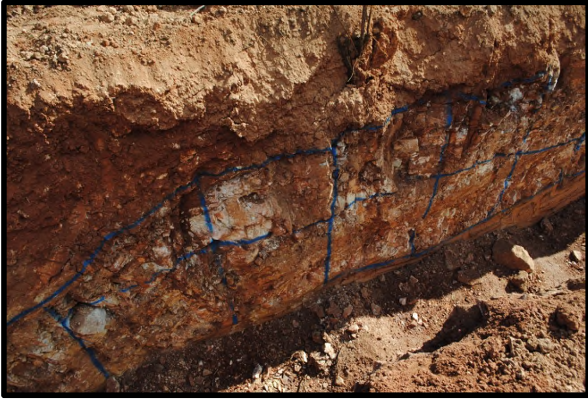
Costeans at Northern Star/St Pats – Costean is near 3m deep. Quartz is near 0.5m thick
