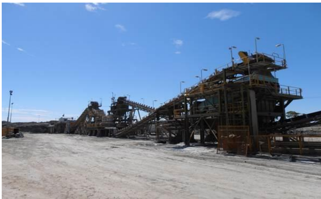
Figure 3: SGM heap leach 3 stage crushing and screening plant (courtesy SGM)
