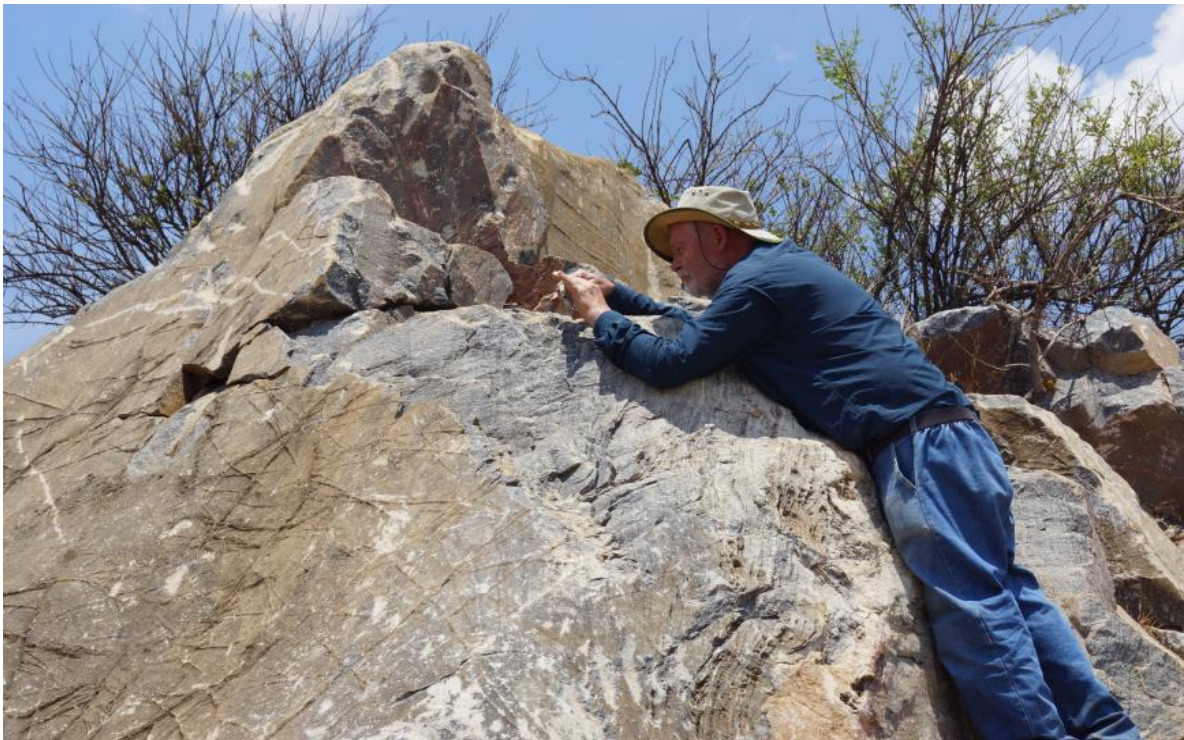
Figure 2: Geologist Robert Barnett at site – this quarry has been mined to 10 metres depth for road base – sampling shows it contains cement grade limestone and that the mineralisation is open in all directions.
