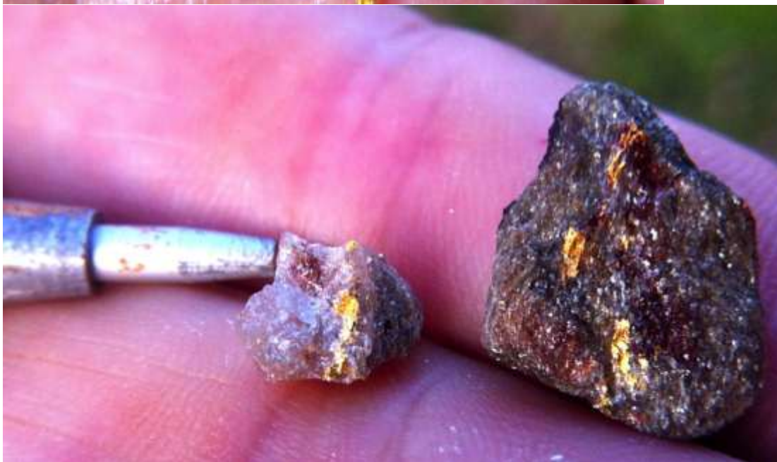
Figures 2a and 2b – Show coarse visible gold up to 5mm strongly elongated parallel to the stretching lineation.
