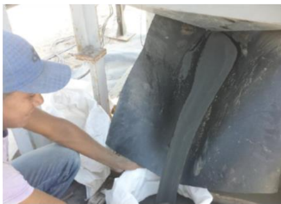
Figure 5 – Magnetite concentrate being bagged from the pilot plant equipment in Peru.
