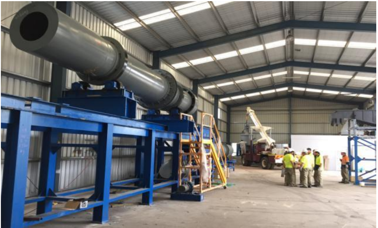
Image 1: Proppant manufacturing pilot plant at Clontarf in Queensland showing external bag houses positioned in place.
