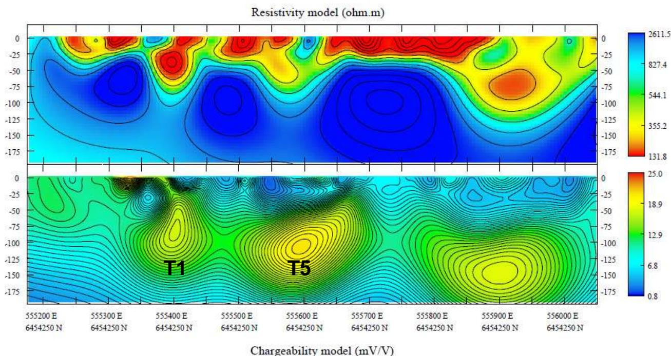
**Figure 3.** Results of ground IP survey along middle traverse on Figure 2 showing the chargeability anomalies that may represent disseminated sulphide at Targets T1 (Red Hill mine) and Target T5).
