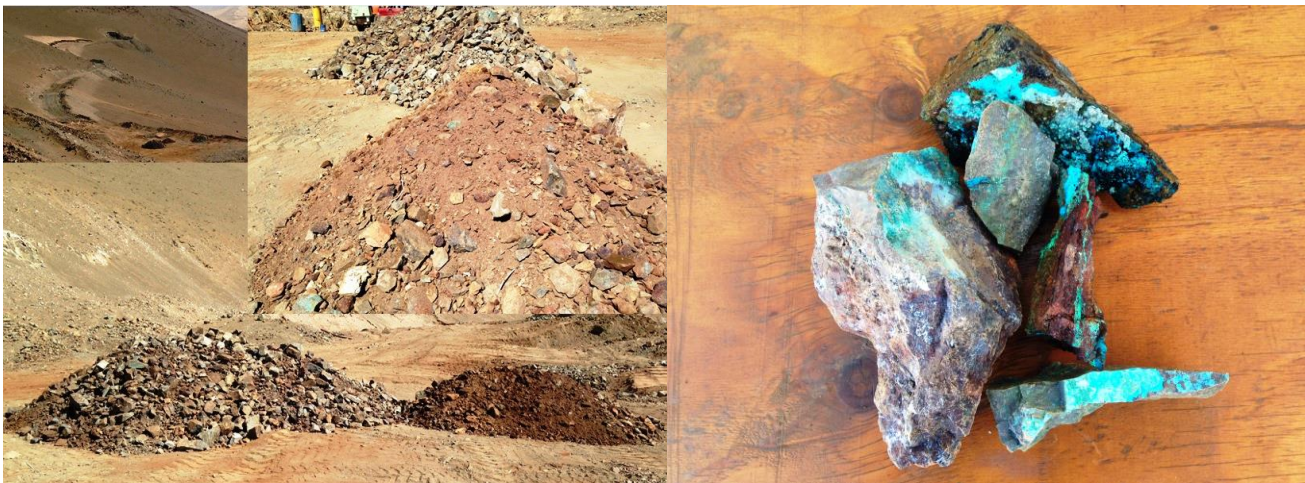
Figure 1- Left) Stockpiled high grade ore from the Viuda vein 1005 Level, right) samples of high grade copper ore from the Viuda vein 1005 Level.
