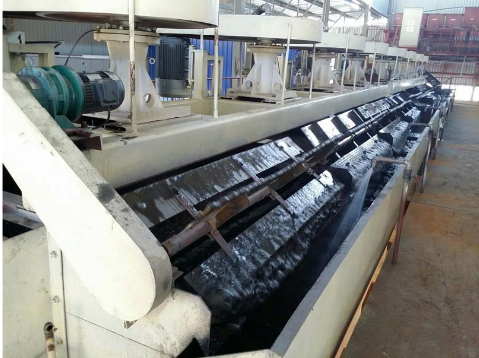
Photograph; Flotation cells in operation at Lubuk Mandi as the first stage of concentrating gold from existing tailings for recovery.
