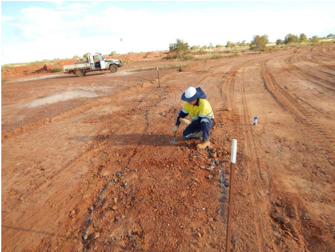
Figure 4. Uncovering never before exposed quartz veins in central zone of Old Pirate (quartz boundaries marked with blue paint lines)
